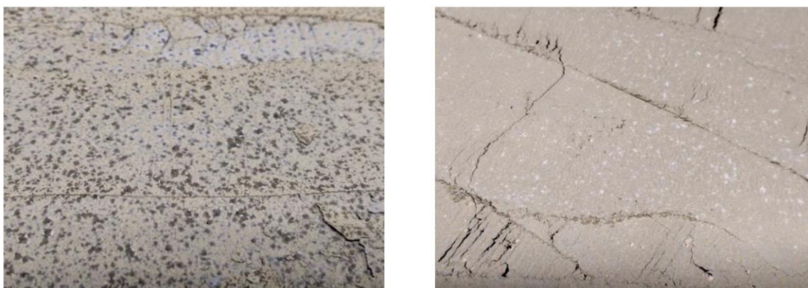
Fig. 8: Surface discolourations of the model SLU formulation (left) and of pure PC (right), appearing when aged with citrate at 35\text{ }^\circ\text{C} and 90\text{ \% RH} .
