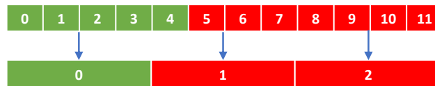
Figure 7.2.: Representation of the computation of a block of target labels, where each bottom block corresponds to 4 source timesteps. The green color indicates a label of L (Low confinement) while red represents H mode. A majority of the labels in the source timesteps 4 - 7 are in H mode, so the corresponding block at target timestep 1 is labeled as H.
