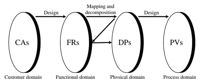
Fig. 2. The four domains of Axiomatic Design [8].
