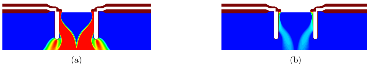
Figure 7.13: Close-up view of the front side of the device depicting (a) the electric current density shortly before device latch-up and (b) the corresponding Auger recombination rate. The emitter-side injection of electrons as well as the increased carrier recombination rates due to the high carrier densities alongside the line of injection are clearly visible.
