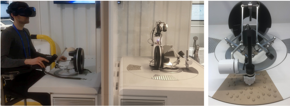
Figure 5.1: Mobile World Congress teleoperation setup based on augmented force feedback haptic devices. The operator is able to explore the remote environment and gets thermal, force, and tactile feedback.
