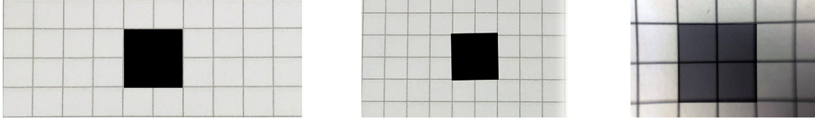
Figure 4.4: Well-defined squared patterns for the identification of maximum coarse texture element sizes. A structural element of 10 \text{ mm}^2 is 240 - 300 pixel large given the usual recording distance of 100 \text{ mm} - 140 \text{ mm} and 4\text{K} resolution. Magnified images (right) are about 1700 pixel at a fix recording distance of 25 \text{ mm} . These values are relevant to determine appropriate sizes of image feature parameters, notably, the coarseness feature. Also note that these parameters help in determining the relevant image size for deep learning-based image classification in Section 4.5. If coarse materials occupy 300 pixels in width and height, and if an overlap of 100 pixels is considered for data generation, an overall width/height of 500 pixels is chosen as image patch input size.
