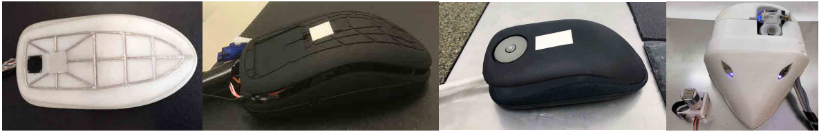
Figure 5.2: Tactile computer mouse evolution. The first version (left) and two improved design versions [5] (middle-left and middle right) are able to display the five relevant tactile dimension from [63] either using an embedded VCA or a C2 tactor, respectively. The current version TCM2 (right) is further able to recreate the fifteen subdimensions from Fishel et al. [66].
