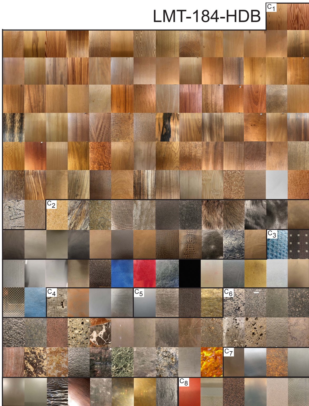
Figure 3.3: Final haptic material database image montage. The different classes C have been separated by black lines. The class names are C_1 woods, C_2 biodegradables, C_3 plastics, C_4 ceramics, C_5 glasses, C_6 stones, C_7 metals, C_8 composites. The class imbalance toward woods actually reflects the true circumstance that this class has the most real world representatives, i.e., types of trees (adapted from [2] © 2019 IEEE).
