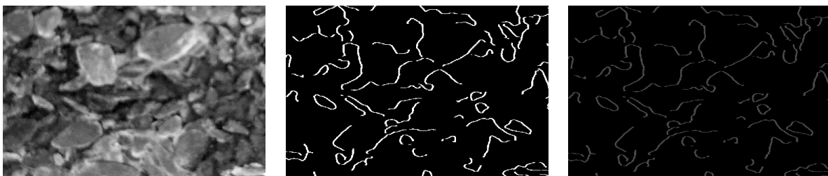
Figure 5.13: Tangential macroscopic roughness image generation I_{\text{macro,tang}} . The grayscale converted surface images provide the positions of laterally-perceivable edges (left). A Canny edge detector (threshold = 0.33, sigma = 4) identifies relevant edges and a dilation filter (middle) broadens the edge width. The value range of the IR sensor data, normalized between 0 and 1, is then used to set the intensity of the dilated edges (right) and thereby determines the intensity of the tangential obstacle (adapted from [5] © 2018 IEEE).
