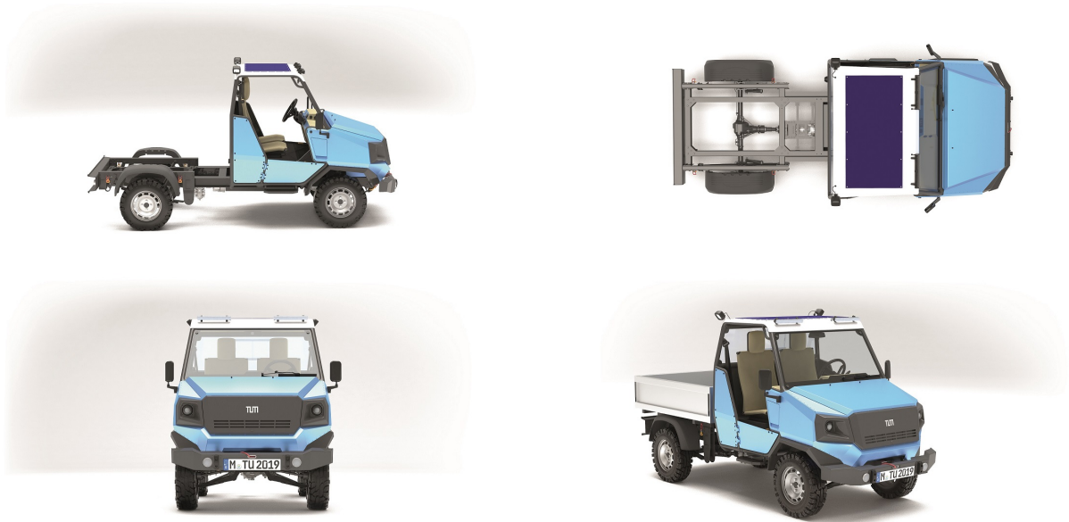
Figure 1.3: Side view (top left), top view (top right), front view (bottom left) and side view with cargo superstructure (bottom right) of the aCar.
