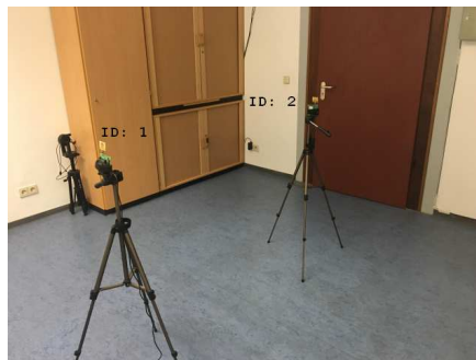
Figure 7. The measurement setup consist of two transceivers (EVK100) with the identification number 1 and 2.
