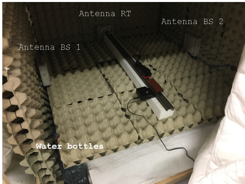
Figure 3.7.: Interference test for the second box
