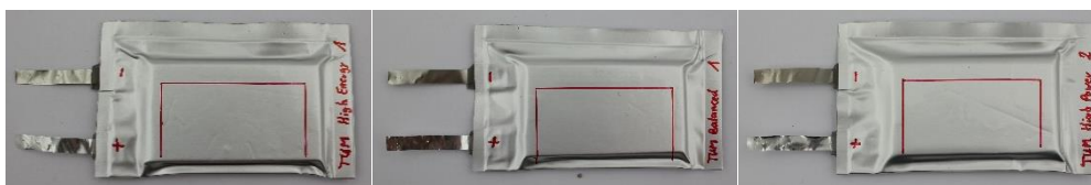
Figure 90 Neutron diffraction sample cells, High Energy (HE), Balanced (BA) and High Power (HP). The red square marks the area where the cell is free from adhesive tape. Image reprinted from [191].
