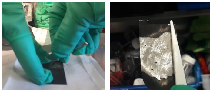
Figure 49 Mechanical removal of active material from double-coated LFP cathode (left). Electrode with removed backside and lightly damaged current collector (right). Glovebox work Jörn Wilhelm. Image taken by K. Wachutka reprinted from [158].
