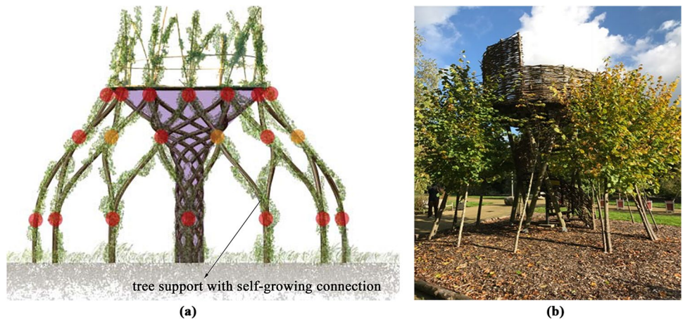
Fig. 6 Self growing structures, a design concept of self-growing structures (dots represent locations of self-growing connections), b existing self-growing structures in the Botanical Garden at TU Delft
