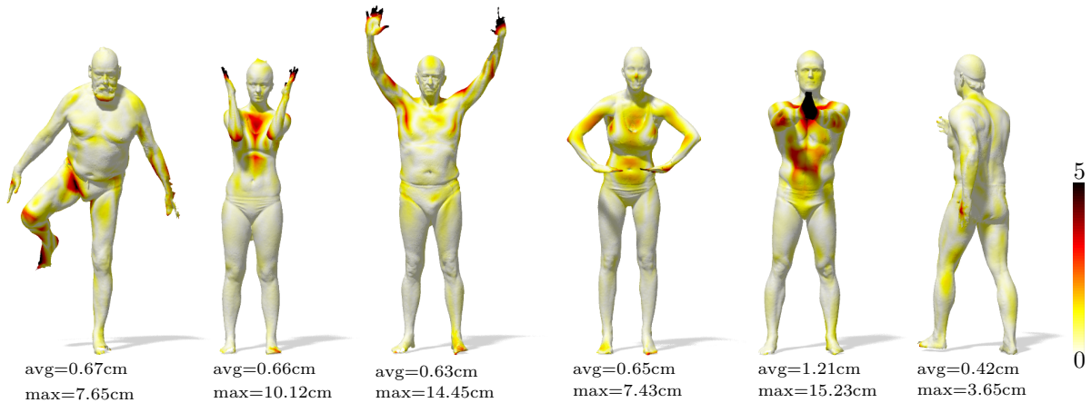
Figure 10.6: Example registrations from the FAUST scan data set. The surface color corresponds to the Euclidean surface distance between scan and registration. The scale of the scans is in real cm values and the same on all plots. We report the average and maximum error under each image. Many errors occur due to the SHOT descriptors being corrupted at holes and in noisy areas (e.g. the hands). Furthermore, in some case the assumption of exact volume preservation is too restrictive for real scans with noise and topological changes (see especially second to the right).
