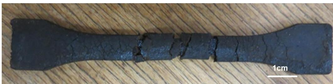
**Figure 3.13:** *Chitin/lignin composite material (CL\_3) fabricated by melt compounding.*
