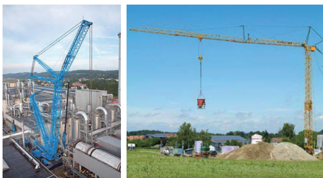
Figure 1. A typical crawler crane and a fast-erecting tower crane (Citation: Liebherr)
