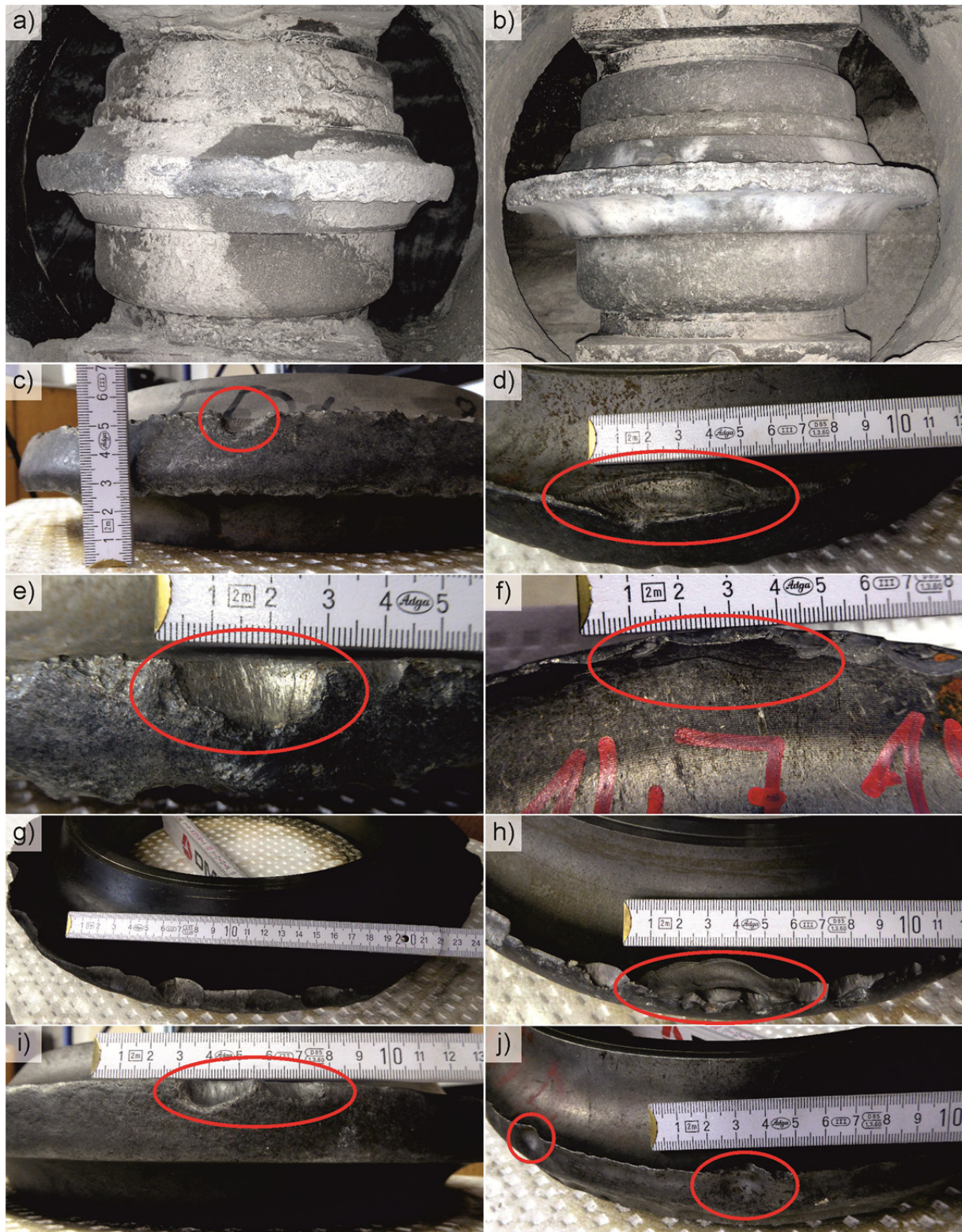
Fig. 63: TBM disc cutters showing types of mushrooming and chipping.
