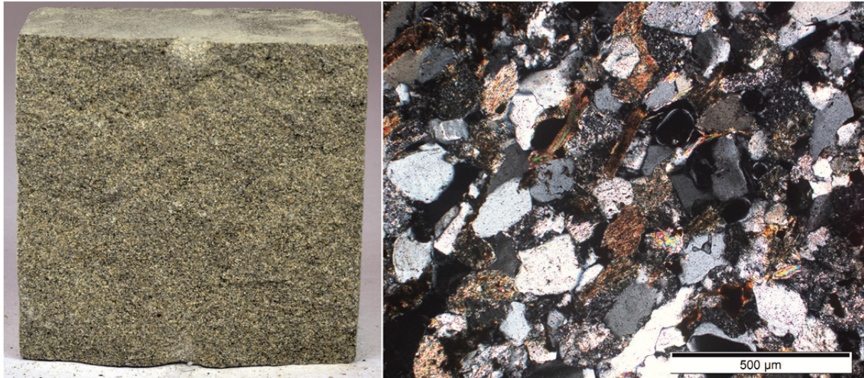
Fig. 37: Left: fine-grained Abtswind Sandstone Castell (cube width = 5 cm); right: microscopic photo with mainly quartz, minor clay minerals, feldspar and lithoclasts (X-pol).
