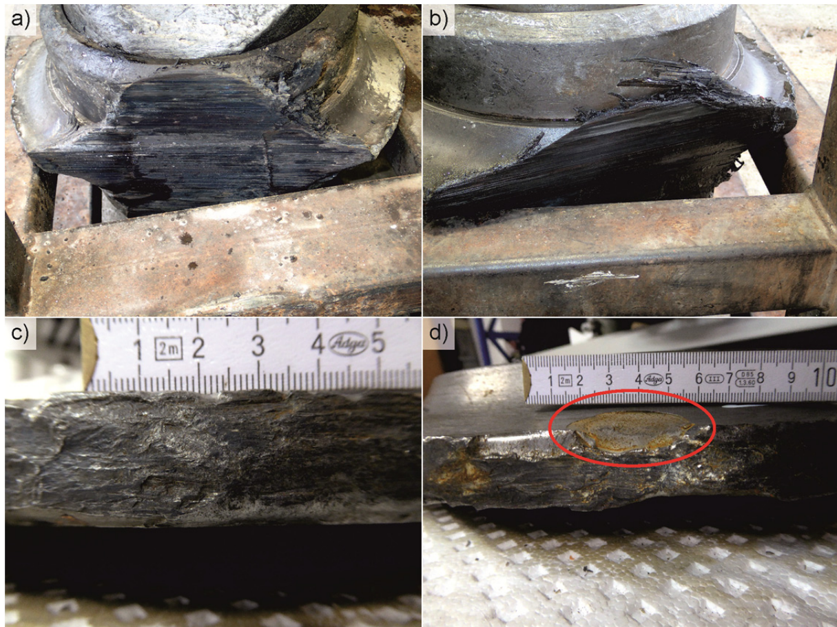
Fig. 66: TBM disc cutters showing blockage damage.
