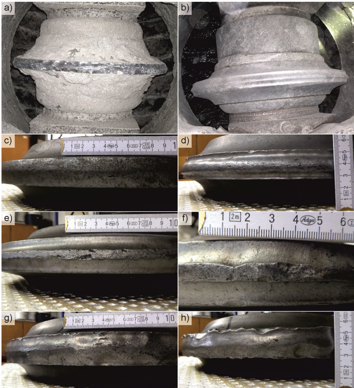
Fig. 64: TBM disc cutters showing types of tapering and sometimes grooving. a) Tapering during operation b) Tapering with grooving during operation c) Tapering d) Asymmetric tapering with grooving e) Tapering with grooving f) Close-up tapering with grooving g) Tapering with grooving and little mushrooming and chipping h) Tapering with grooving, mushrooming and chipping.
