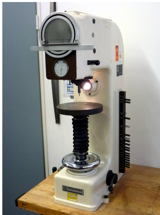
Fig. 58: The universal hardness tester DIA TESTOR, model 2 Rc manufactured from Wolpert in 1958 was used for the Rockwell hardness tests, the Vickers hardness tests and the modified Vickers hardness tests.
