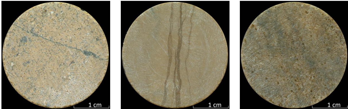
Fig. 51: Left: limestone (ooidal, fossiliferous grainstone (2,895 mTVD)); middle: dolomitic limestone (mudstone (3,055 mTVD)); right: medium crystalline dolostone (3,154 mTVD).
