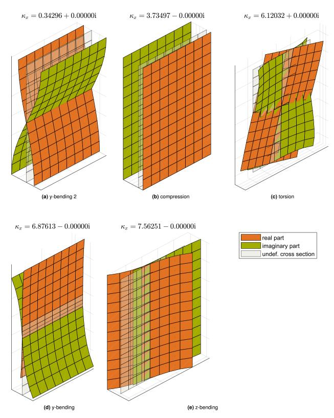
Figure 2.8: Eigenvectors belonging to real-valued wavenumbers of the rectangular concrete cross section at  $2000 {\rm Hz}$
