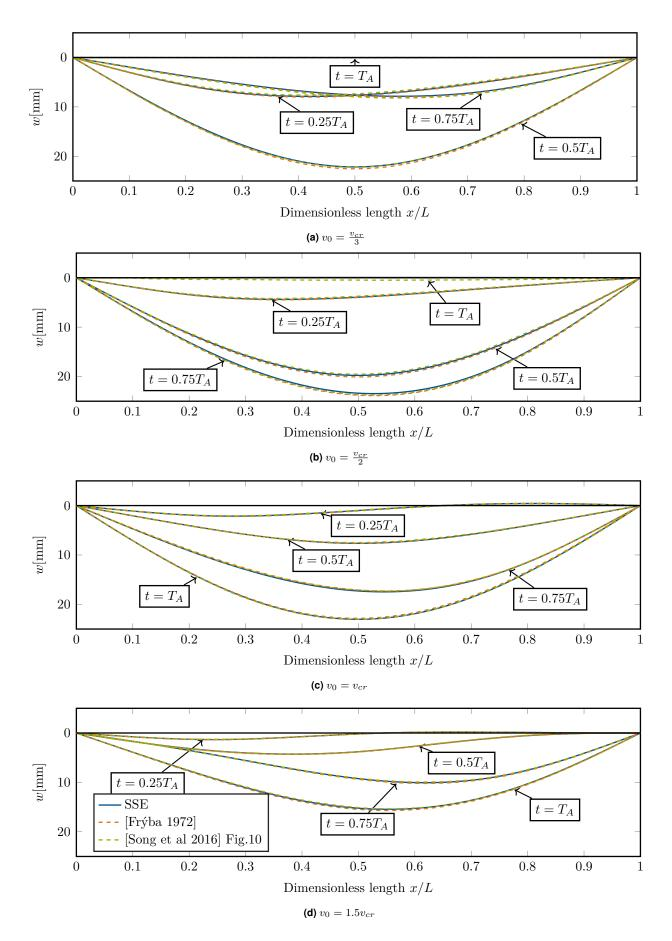
Figure 4.12: Time-dependent vertical deflection of the single-span beam subjected to a moving force with different constant velocities  $v_0$ . The solution of the SSE model is compared to two reference solutions from literature.
