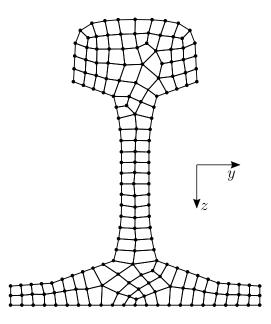
Figure 2.1: Exemplary cross-sectional mesh of four-noded elements
