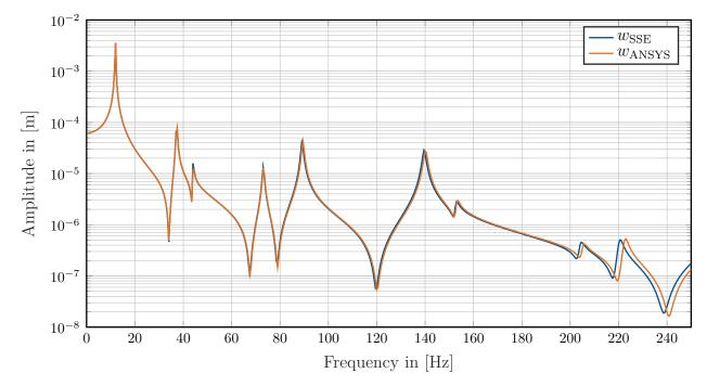
Figure 3.16: Harmonic analysis of the 14m two-span concrete beam loaded with a single force  $F_z = 1kN$  at x = 10m. Mean value of the amplitudes of the *w*-deflections at the excitation nodes. Loss factor  $\eta = 0.01$ . Frequency range: 1-250Hz
