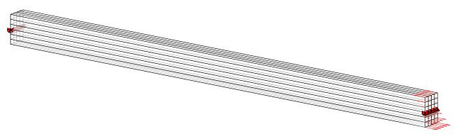
Figure 3.2: SSE model of a single span concrete beam (L = 10m) with bearings and loads
