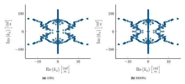
Figure 2.4: Wavenumbers of the rectangular concrete cross section in complex plain
