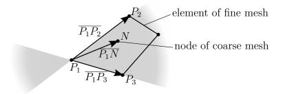
Figure 5.1: Vectors used in the cross product test. The test is positive if the considered Node N is in the gray area.
