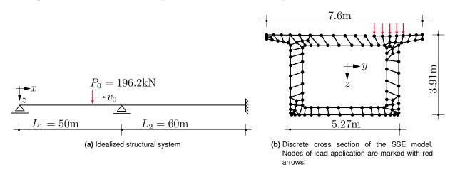
Figure 4.15: SSE model of the Filstal bridge
