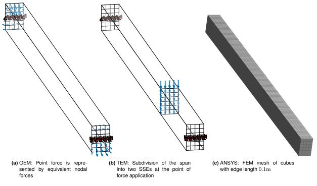
**Figure 4.5:** Models for a 10m single-span beam loaded with a point force  $P_0 = 1$ kN at x = 3m (from [Mader 2019])
