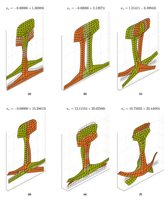
Figure 2.15: Eigenvectors belonging to the lowest magnitude complex-valued wavenumbers of the UIC60  $_{rail\,cross\,section\,at\,100Hz}$
