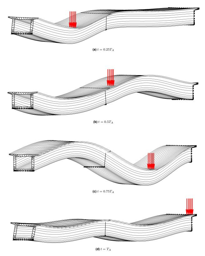
**Figure 4.19:** Deflection shapes of the considered section of the Filstal bridge under a moving load with  $v_0 = 288 \frac{\text{m}}{\text{s}}$  at different times *t*. Number of DFT samples:  $N = 2^8$
