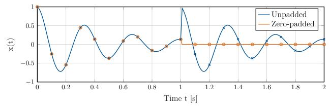
Figure 4.8: Zero padding used to cope with the wraparound error
