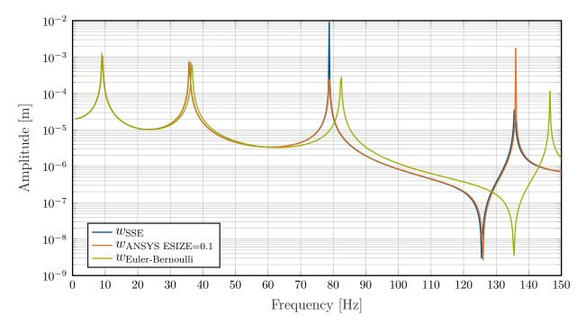
Figure 3.6: Harmonic analysis of the 10m single span concrete beam loaded with a section moment  $M_y = 1$  kNm at x = 10m. Mean value of the *w*-deflection of all cross-sectional nodes at x = 2.6m. Frequency range: 1-150Hz
