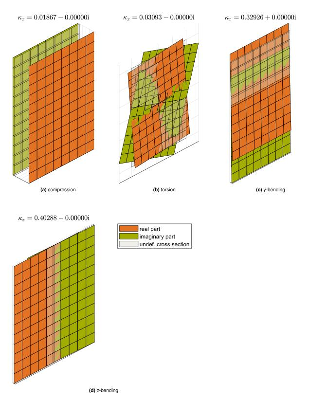
Figure 2.7: Eigenvectors belonging to real-valued wavenumbers of the rectangular concrete cross section at  $10 {\rm Hz}$
