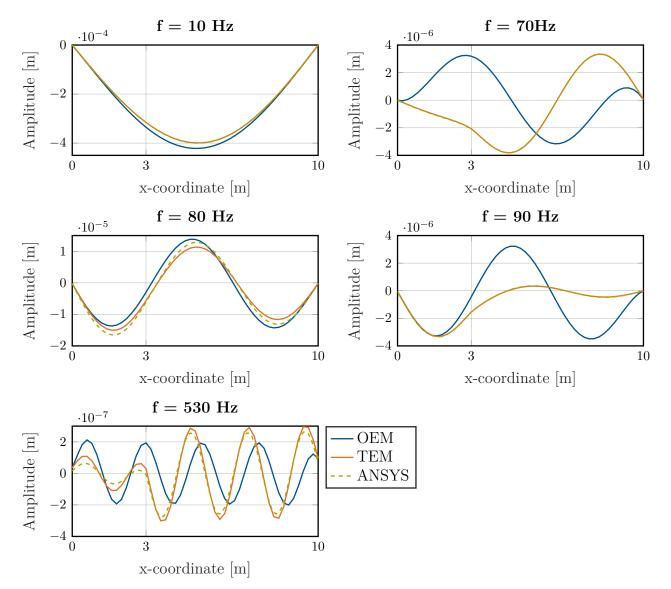
**Figure 4.7:** Mean value of the vertical deflection (*z*-direction) of the cross-sectional nodes of the singlespan beam modeled as OEM, TEM and with finite elements plotted over the longitudinal *x*-axis at different frequencies
