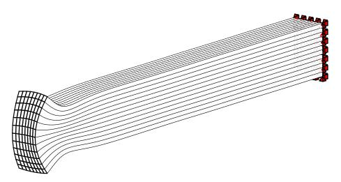
Figure 5.11: Deflection shape of the concrete cantilever beam at 2480Hz. Resonant response with a cross-sectional mode at the free end.
