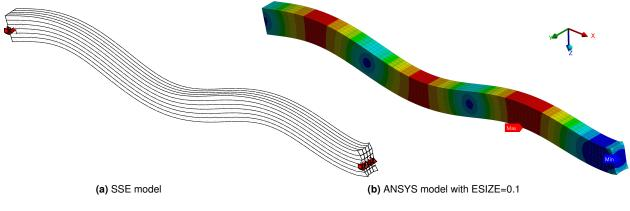
Figure 3.4: Deformation shapes of the single span concrete beam at  $100 \mathrm{Hz}$
