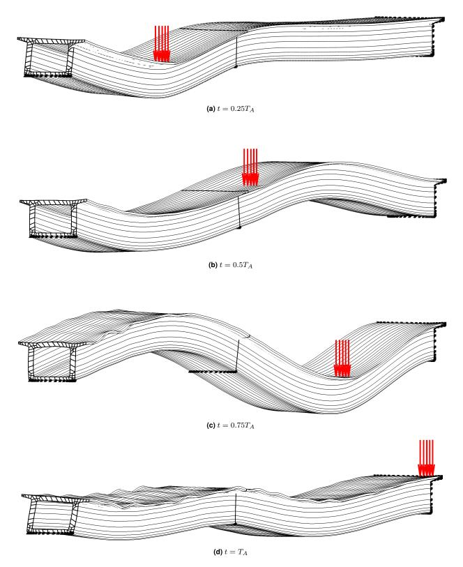
**Figure 4.20:** Deflection shapes of the considered section of the Filstal bridge under a moving load with  $v_0 = 288 \frac{\text{m}}{\text{s}}$  at different times *t*. Number of DFT samples:  $N = 2^7$
