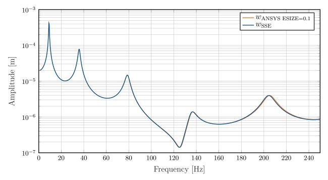
Figure 3.8: Harmonic analysis of the damped ( $\eta = 0.05$ ) 10m single span concrete beam loaded with a section moment  $M_y = 1$ kNm at x = 10m. Mean value of the *w*-deflection of all cross-sectional nodes at x = 2.6m. Frequency range: 1-250Hz
