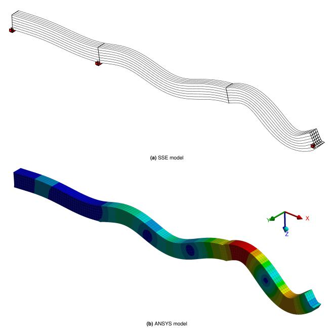
Figure 3.15: Deformation shapes of the multi-span concrete beam at  $180 \mathrm{Hz}$
