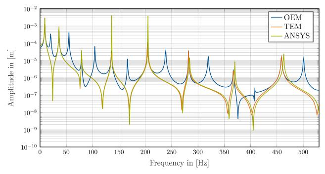
Figure 4.6: Frequency response of the single-span beam modeled as OEM, TEM and with finite elements. Mean value of the magnitude of the nodal deflections at the point of load application (x = 3m)
