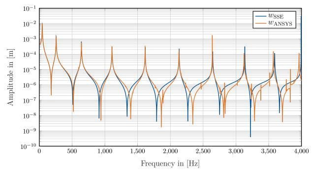
Figure 3.12: Harmonic analysis of the 2m cantilever UIC60 rail section loaded with a single force  $F_z = 1 \text{kN}$  at x = 2m. Amplitude of the *w*-deflection of the evaluation node specified in Fig. 3.9. Frequency range: 2-4000Hz
