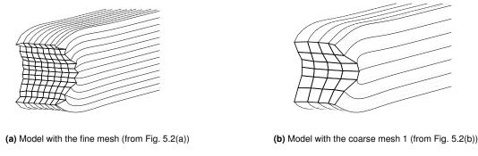
Figure 5.8: Deflection shapes of the concrete cantilever beam at 1600 Hz
