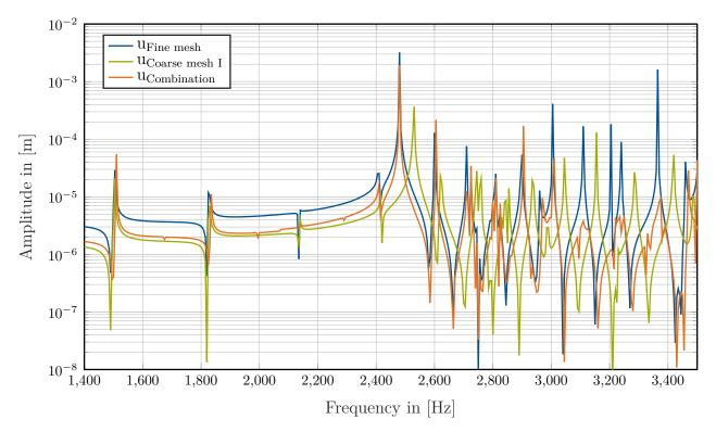
**Figure 5.6:** Harmonic analysis of the 5m cantilever concrete beam loaded with a stepped force pattern at the free end. *u*-deflection of the center node at the free end. Three different cross-sectional discretizations: Original SSE formulation with the fine mesh from Fig. 5.2(a) and with the coarse mesh I from Fig. 5.2(b) and the proposed enhanced displacement ansatz with a combination of both meshes.
