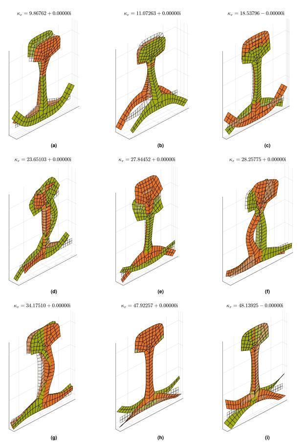
Figure 2.14: Eigenvectors belonging to the real-valued wavenumbers of the UIC60 rail cross section at  $\rm 10000 Hz$
