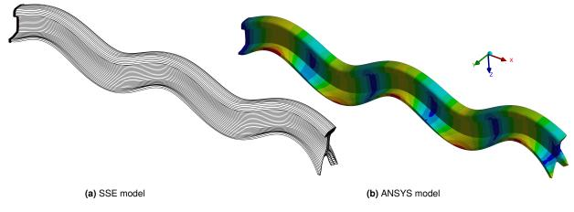
Figure 3.11: Deformation shapes of the cantilever UIC60 rail at 2000 Hz
