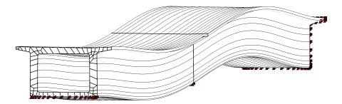
Figure 4.16: Deformation of the bridge model loaded with a section moment  $M_y$  at x = 0m at 3.340Hz. Approximated first mode shape.
