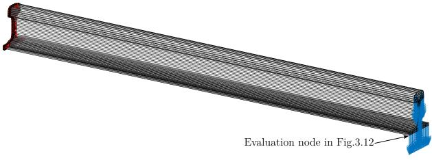
Figure 3.9: SSE model of a UIC60 rail section (L = 2m) with bearings and loads
