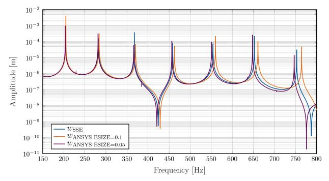
Figure 3.7: Harmonic analysis of the 10m single span concrete beam loaded with a section moment  $M_y = 1$  kNm at x = 10m. Mean value of the *w*-deflection of all cross-sectional nodes at x = 2.6m. Frequency range: 150-800Hz
