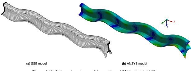
Figure 3.13: Deformation shapes of the cantilever UIC60 rail at 2,468Hz
