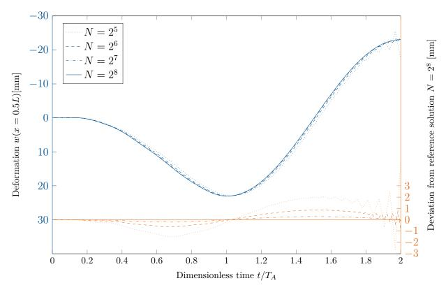
Figure 4.10: Convergence study for the single-span example loaded with a moving force with the lowest critical velocity  $v_{cr}$  (similar to [Mader 2019]). Vertical deflection in the middle plotted over the dimensionless time for different numbers of DFT samples N.
