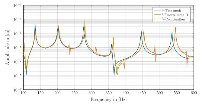
**Figure 5.4:** Harmonic analysis of the 10m single span concrete beam loaded with a section moment  $M_y = 1$ kNm at x = 10m. Mean value of the *w*-deflection of all cross-sectional nodes at x = 2.6m. Three different cross-sectional discretizations: Original SSE formulation with the fine mesh from Fig. 5.2(a) and with the coarse mesh II from Fig. 5.2(c) and the proposed enhanced displacement ansatz with a combination of both meshes.
