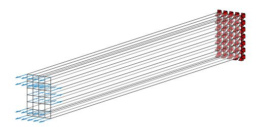
Figure 5.5: SSE model of a concrete cantilever beam (L = 5m) with bearings and loads
