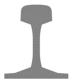
Figure 3.10: Cross section at x = 2m of the ANSYS model for the UIC60 rail
