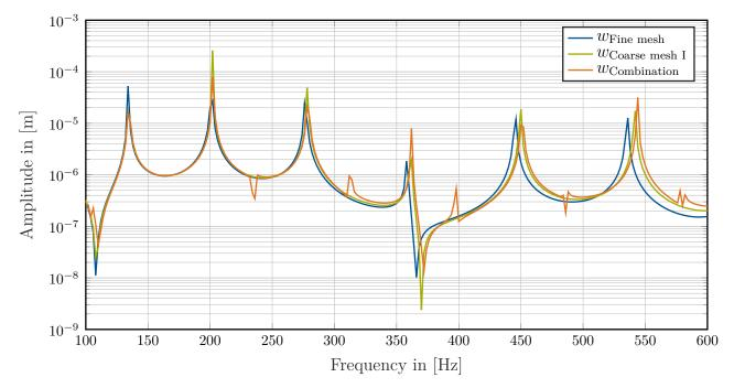
**Figure 5.3:** Harmonic analysis of the 10m single span concrete beam loaded with a section moment  $M_y = 1$ kNm at x = 10m. Mean value of the *w*-deflection of all cross-sectional nodes at x = 2.6m. Three different cross-sectional discretizations: Original SSE formulation with the fine mesh from Fig. 5.2(a) and with the coarse mesh I from Fig. 5.2(b) and the proposed enhanced displacement ansatz with a combination of both meshes.
