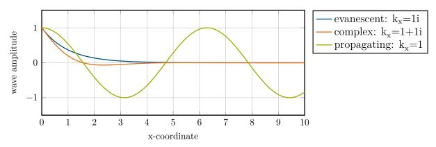
Figure 2.6: Exemplary visualization of an evanescent wave, a wave with complex valued wavenumber and a propagating wave
