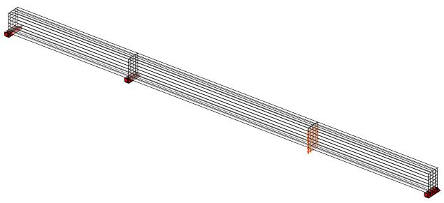
Figure 3.14: Undeformed SSE model of the two-span concrete beam with supports at x = [0,4,14]m and vertical load application at x = 10m
