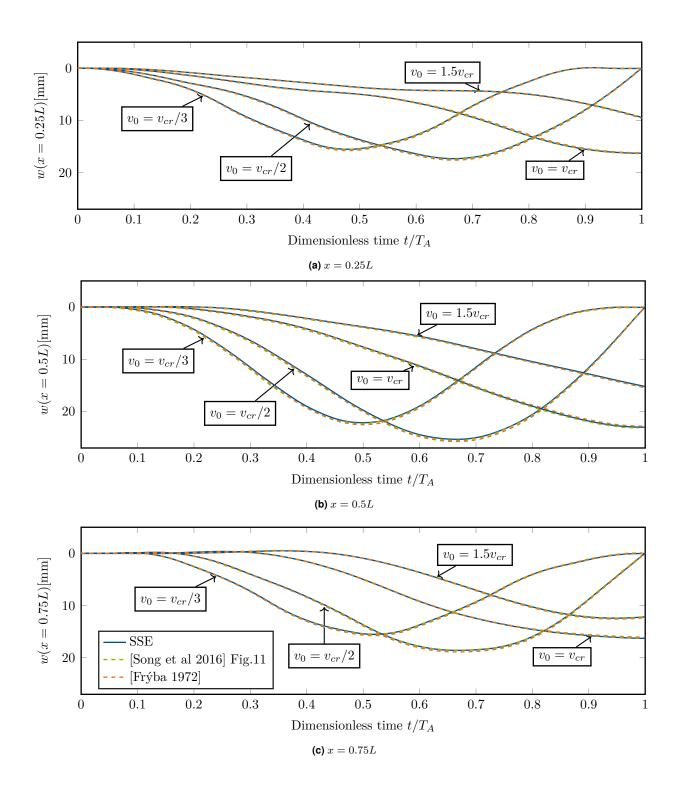
**Figure 4.13:** Vertical deflection at tree different *x*-coordinates of the single-span beam subjected to a moving force with different constant velocities  $v_0$ . The solution of the SSE model is compared to two reference solutions from literature.
