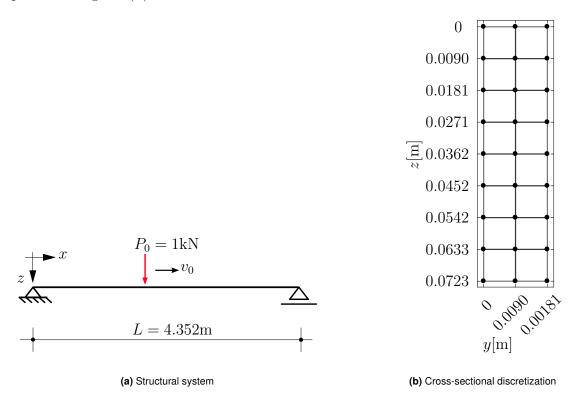
Figure 4.9: Structural model of a single-span rectangular beam under a moving force
