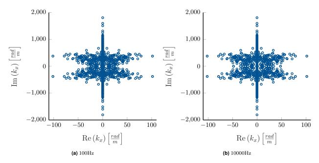
Figure 2.11: Wavenumbers of the UIC60 cross section in complex plain
