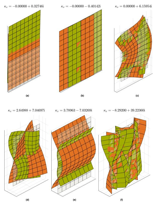
Figure 2.9: Eigenvectors belonging to complex-valued wavenumbers of the rectangular concrete cross section at  $10 \rm Hz$
