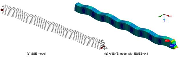
Figure 3.5: Deformation shapes of the single span concrete beam at  $700 \mathrm{Hz}$
