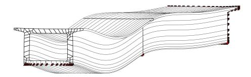
Figure 4.17: Deformation of the bridge model loaded with a section moment  $M_y$  at x = 0m at 4.805Hz. Approximated second mode shape.
