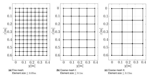
**Figure 5.2:** Cross-sectional meshes considered in this example
