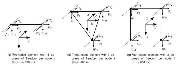
Figure 1.2: Finite elements used in literature for the discretization of the cross section
