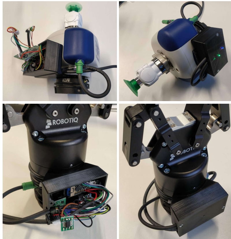
Figure 8.12: Custom Wi-Fi OPC UA tool device adapter based on the TinyPICO Microcontroller board with FreeRTOS. The only external connection required is a 24 V power supply.
