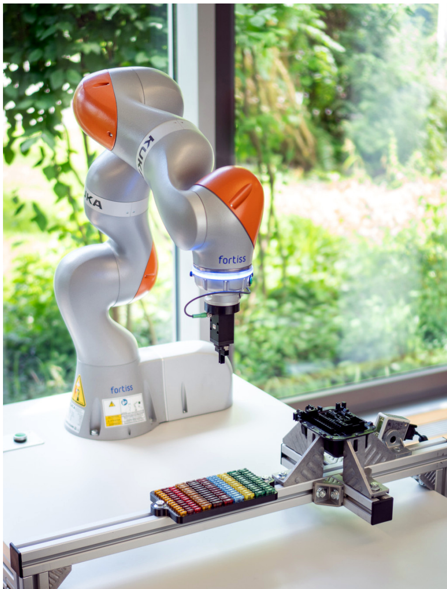
Figure 7.7: System setup for Knowledge-based fuse insertion build upon my proposed Plug & Produce architecture.
