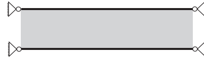
FIG. 2. Modeling of simply supported boundary conditions by constraining the displacement DOFs of the face sheet edges.
