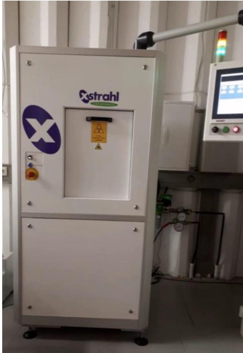
Figure 8: X Strahl RS225 radiation machine as used in the Research Unit Medical Radiation Physics and Diagnostics at Helmholtz Center Munich.
