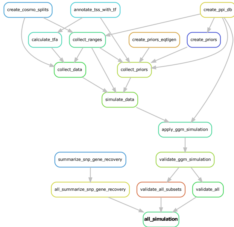
Figure 3.2.: Example ‘rule graph’ for the Snakemake pipeline when executing the network inference simulation study. Graph was created using the snakemake -rulegraph command. Individual nodes are rules and edges reflect dependencies between the rules. When the target rule (bold) is called, Snakemake identifies all dependencies and builds an instance of the workflow.
