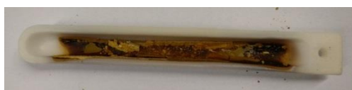
Figure 5.4: Residues in the corundum boat after fluorination, identified as \text{MoF}_3 by XRPD (also see Figure A.5).
