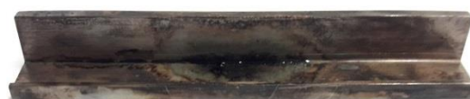
Figure 6.3: Residues of ruthenium after being exposed to the lab atmosphere for 15 minutes.
