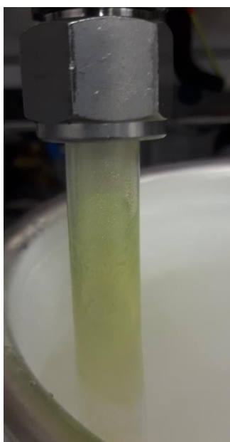
Figure 6.6: Reaction product of the fluorination of ruthenium in the first cold trap, which was cooled using \text{LN}_2 . The deposition is of emerald green color, suggesting it to be \text{RuF}_5 .
