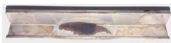
Figure 6.16: Palladium powder after being exposed to the lab atmosphere for seven minutes. A thin, colorful film deposits on the Monel carrier.
