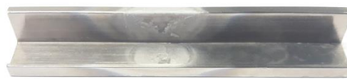
Figure 5.19: Residues after fluorination at a \text{NF}_3 flow of 35 sccm with complete consumption of the uranium target. The white powder is \text{AlF}_3 as shown by XRPD.
