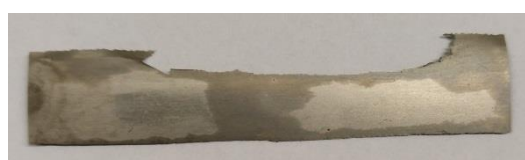
Figure 6.19: Tungsten sheet after fluorination for 35 minutes.
