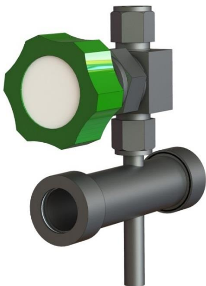
Figure 4.27: CAD model of the measuring cell used for acquisition of IR and UV/VIS spectra.
