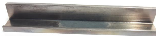
Figure 6.34 Residues of the osmium after being exposed to the plasma for 75 minutes. Mass of the residues equal to 6.6 mg, accounting for a reaction yield of about 97 %.
