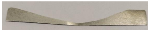
Figure 5.3: Molybdenum sheet after fluorination for 55 minutes at 300 W with a mass 298.3 mg.
