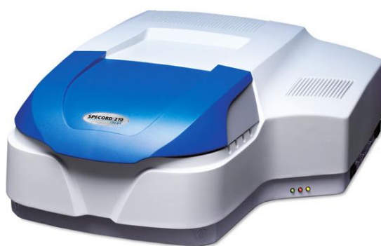
Figure 3.4: The double-beam photometer SPECORD 210 PLUS as used for all UV/VIS measurements, covering the wavelength region from 190 to 1100 nm.
