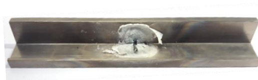
Figure 5.25: Residues after fluorination at a \text{NF}_3 flow of 25 sccm.
