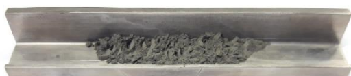
Figure 6.42: Iridium powder on the Monel boat before fluorination. The applied mass in this picture amounts to 722.3 mg.
