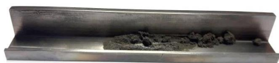
Figure 6.53: Platinum powder after fluorination for 150 minutes at an elevated temperature of 190 °C. Although there is no change in appearance under the microscope, the powder agglomerates much easier.
