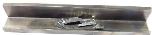
Figure 6.65: Tellurium chunks on a Monel boat before fluorination. Total mass of this sample is 552 mg.
