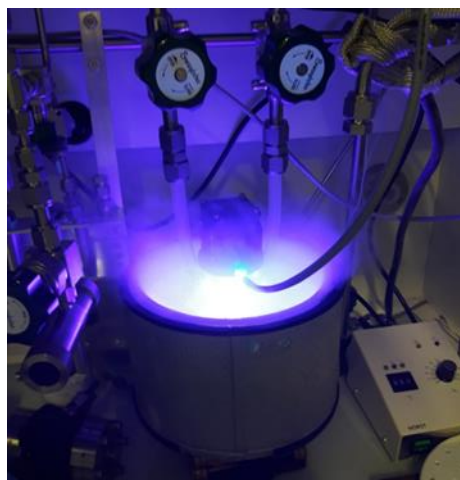
Figure 5.46: Investigation of the reaction of \text{MoF}_6 and \text{UF}_6 with liquid CO at a temperature of 75 K under irradiation at a wavelength of 395 nm.
