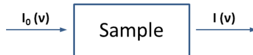
Figure 3.6: The physical principal of IR transmission spectroscopy. The incident beam with the intensity I_0 excites transitions between vibrational levels and is thereby attenuated to the intensity I [62].
