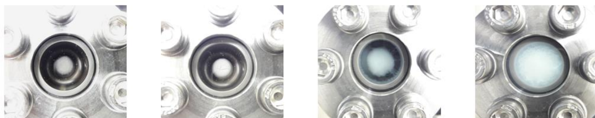
Figure 5.50: View from above into the high-pressure container during the UV irradiation. From left to right: (1) white UF 6 /MoF 6 mixture sublimed at the cold finger in the center of the chamber; (2) after venting the container with supercritical CO; (3) after irradiation for 7 minutes and (4) after irradiation for 60 minutes.
