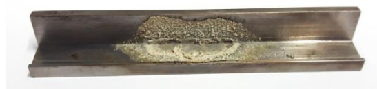
Figure 6.2: Residues of ruthenium after fluorination for 100 minutes at an elevated temperature of 190 °C.
