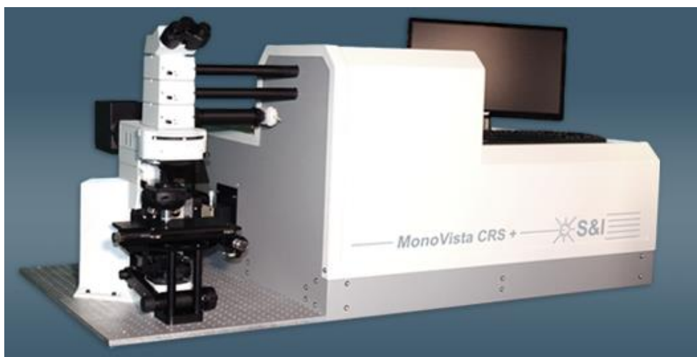
Figure 3.13: The MonoVista CRS+ as used for the acquisition of all Raman spectra measured during the experiments [84].
