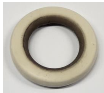
Figure 2.10: FFKM O-ring made from Perlast G75H without any signs of degradation after \text{NF}_3 plasma exposure at a temperature of 210 °C for 2 hours. The black deposits show to be removable.
