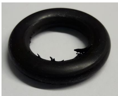
Figure 2.9: FFKM O-ring made of Parofluor V8920-75 showing clear signs of degradation after \text{NF}_3 plasma exposure at a temperature of 200 °C for 2 hours.
