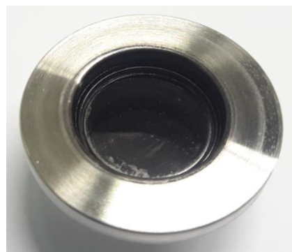
Figure 4.17: Sapphire window after being used for approximately 100 hours of fluorination.
