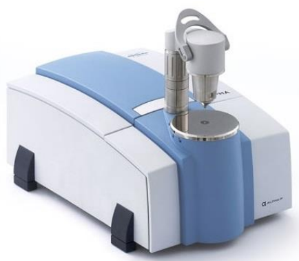
Figure 3.10: The Bruker Alpha , as used for all ATR IR measurements performed during the experiments [81].
