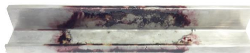
Figure 6.43 Residues of the iridium after being exposed to the plasma for 62 minutes. Mass of the residues equal to 39.2 mg. They are extremely hygroscopic starting to react immediately with the moisture in the lab atmosphere.
