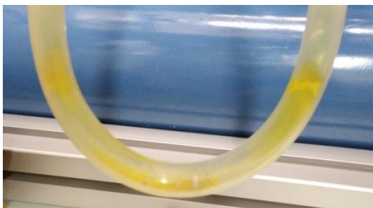
Figure 6.44: Deposited \text{IrF}_6 in the first cold trap using liquid nitrogen as a frigorific agent.
