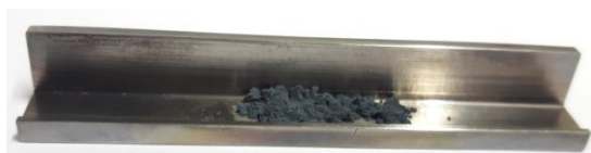
Figure 6.33: Osmium powder on the Monel boat before fluorination. A total mass of 208.6 mg was applied.
