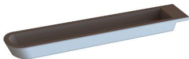
Figure 4.18: CAD model of the corundum boat used in the first set of experiments.
