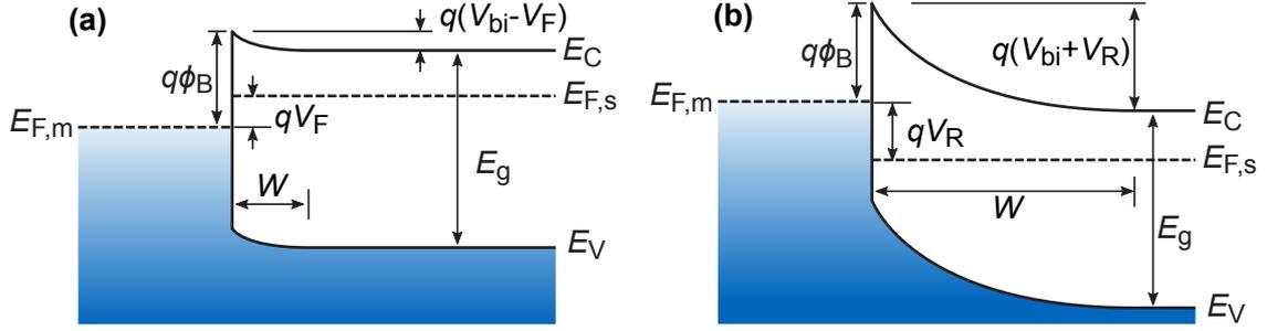
**Figure 2.4:** Energy-band diagrams of a metal-semiconductor contact under different biasing conditions. (a) When a positive (forward) voltage  $V_f$  is applied to the anode (metal) with respect to the cathode (semiconductor),  $E_{F,m}$  is lowered compared to  $E_{F,s}$  and the depletion width gets reduced. A reverse bias  $V_r$  shifts the Fermi levels vice versa and causes a larger  $W$ . Adapted from Ref. [114].
