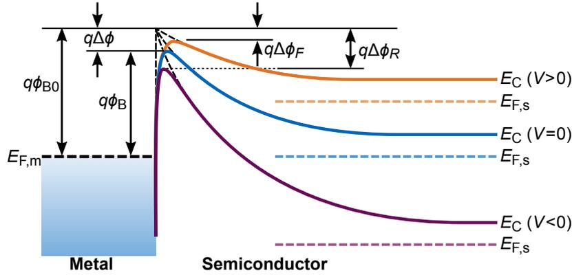
**Figure 2.5:** Energy-band diagrams of a metal-semiconductor contact with barrier lowering at different biasing conditions. The height would be intrinsically  $q\phi_{B0}$  without considering a barrier lowering, but in reality it is lowered by  $q\Delta\phi$  due to an image-force. The magnitude can be altered by applying a voltage to smaller (forward bias) or higher (reverse bias) values, which in turn changes the final barrier height. Adapted from Ref. [114].
