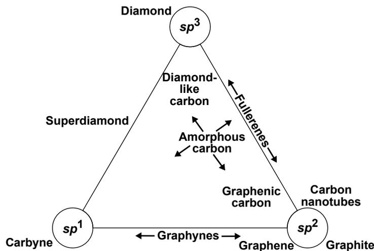
**Figure 1.11:** Ternary phase diagram to describe and classify different carbon allotropes based on their content of  $sp^1$ ,  $sp^2$  and  $sp^3$  hybridized orbitals. Adapted from Ref. [113].
