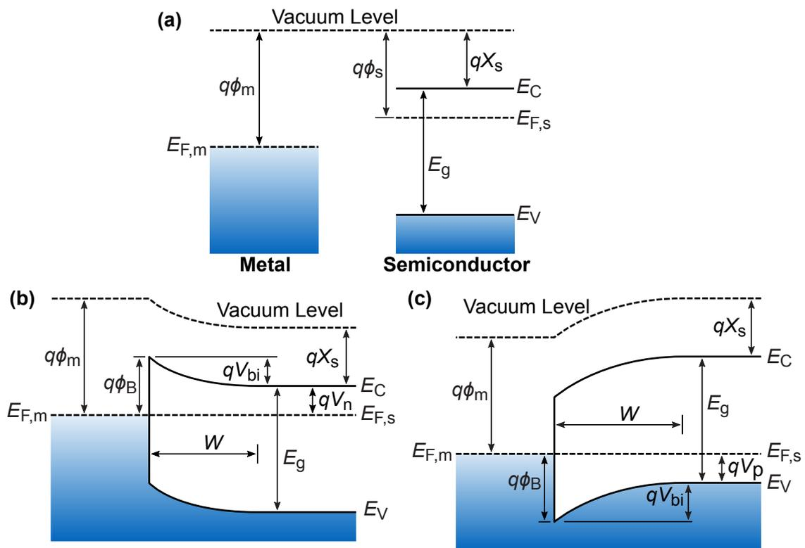
**Figure 2.3:** Energy-band diagrams of a metal-semiconductor system. (a) The metal and the semiconductor are electrically neutral, are still separated from each other and just show an alignment with respect to their vacuum level. The band diagram of an n-type in (b) and p-type semiconductor in (c) with an ideal contact to a metal in thermal equilibrium. The Fermi levels  $E_F$  of the two materials are aligned and the semiconductor bands are bent. Adapted from Refs. [114, 195].
