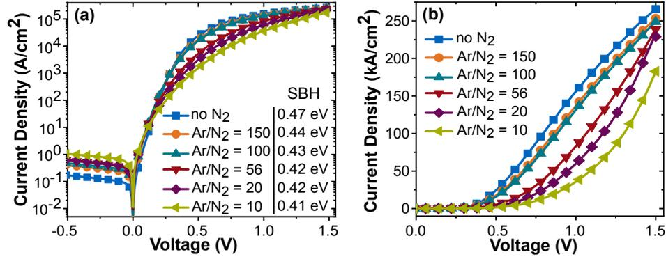
**Figure 4.6:**  $J$ - $V$  curves of CN-Si diodes sputtered at different Ar/N<sub>2</sub> ratios in a semi-log in (a) and a fully linear scale in (b). The diode without N<sub>2</sub> is an SC-Si contact. The thicknesses of all films is in-between 5 nm and 7 nm. A higher content of incorporated nitrogen leads to a lower SBH (the respective values are given in (a) for all diodes) but the forward conduction is less ideal with higher  $R_s$ .
