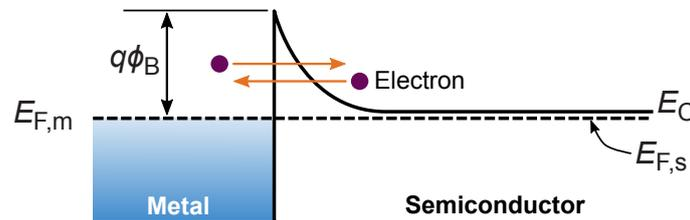
**Figure 2.8:** Energy-band diagram for a metal to a highly doped n-type semiconductor. The depletion region is very small in this case, which leads to a strong band bending. This allows electrons to tunnel through the narrow barrier very easily in both directions.
