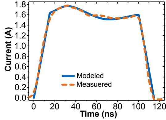
**Figure 2.21:** The modeled waveform in COMSOL in comparison to a real 100 ns long pulse. The modeled one matches with a measured curve. It has the same rise/fall time of 15 ns, a similar overshoot and ‘ringing’ behavior and the same average amplitude level of about 1.6 A (3.5 MA/cm<sup>2</sup>).
