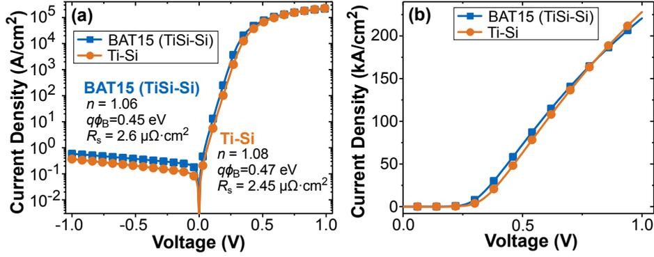
**Figure 4.1:** Comparison of the dc characteristics in a semi-log in (a) and fully linear scale in (b) of a commercial available BAT15 Schottky diode with TiSi-Si and a self-made Ti-Si contact by rf sputtering using the BAT15 test vehicle. Ideality factor  $n$ , SBH  $q\phi_B$  and area-normalized series resistance  $R_s$  are displayed. They are very similar whereas the Ti-Si diode has a higher SBH and ideality factor but a slightly lower series resistance.
