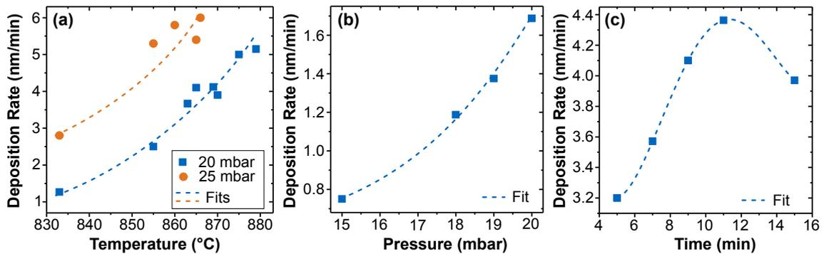
**Figure 3.8:** Carbon deposition rates at different process parameters for  $C_2H_2$  with a gas flow of 20 sccm. (a) Growth rate as function of temperature at a pressure of 20 mbar and 25 mbar. The total time was always between 20 min and 30 min. (b) Deposition rate as function of pressure at 860 °C. (c) Growth rate as function of the deposition time at  $p = 24$  mbar and  $T = 860$  °C.
