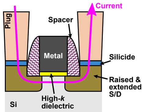
**Figure 1.6:** Schematic current path in a modern FinFET with a raised and extended S/D region. The dimensions, in particular the contact length, are already compressed to such an extent that the current in the silicide essentially has a negligible horizontal component compared to a traditional planar transistor. Therefore, the contact resistance of the silicide to silicon becomes the most important decision criterion. Adapted from Ref. [30].
