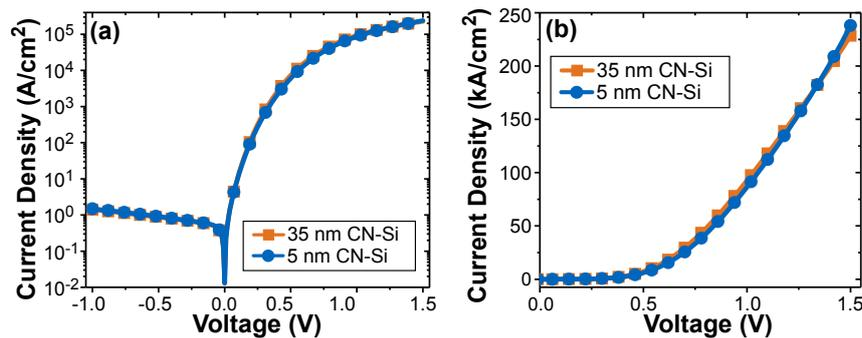
**Figure 4.7:** Comparison of the dc characteristics of CN-Si (400 °C) diodes with 5 nm and 35 nm thick CN in a semi-log in (a) and linear scale in (b). Both curves almost match each other and only the diode with the thinner CN drives more current at a voltage  $\geq 1.5$  V. Taken from Ref. [MS19].
