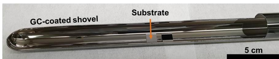
**Figure 3.7:** A photograph of a quartz shovel loaded with two samples, all surfaces are homogeneously coated with 40 nm thick graphenic carbon. It is very shiny with a high reflectivity, but still slightly transparent (hard to recognize here).
