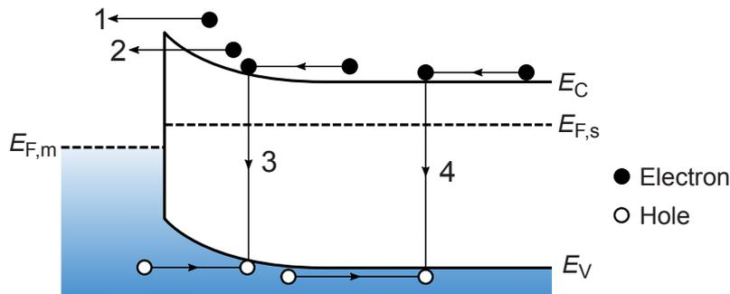
**Figure 2.6:** Energy band diagram of a forward biased Schottky junction on a n-type semiconductor showing four different transport processes. (1) Thermionic emission, (2) tunneling through the barrier, (3) electron-hole recombination in the depletion region, and (4) hole injection from the metal and recombination in the neutral region. Adapted from Ref. [195].
