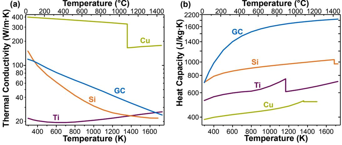
**Figure 2.22:** Temperature-dependent characteristics for the thermal conductivity  $k$  in (a) and heat capacity  $C_P$  in (b) for Si, Ti, Cu and GC. The values are taken from Refs. [249, 250]. A discontinuity in the curve in general indicates a transition from solid to liquid, except for Ti in (b) where only the crystal phase changes.
