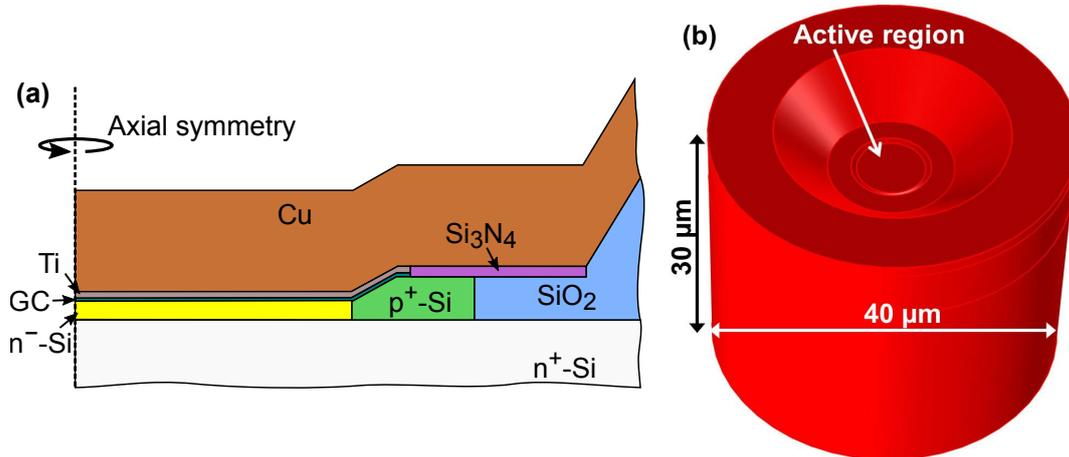
**Figure 2.20:** The geometric model of the BAT15 diode used in FEM simulations. (a) shows a section of the used 2D model of a BAT15 drawn in COMSOL. Geometric variations occur only in radial and vertical, but not in angular direction. The axial symmetry is around the center of the active region. (b) A rotation of the 2D model results in a cylindrical 3D solid. The height is set to  $30\ \mu\text{m}$  and the radius to  $20\ \mu\text{m}$ .
