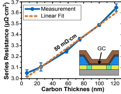
**Figure 4.3:** The area-normalized series resistance of the CVD-C-Si diode  $R_s$  as a function of the graphenic carbon thickness. All tested diodes have similar GC deposition parameters, only the growth time was altered, and the same metallization layers on top. The out-of-plane electrical resistivity is extracted to be 50 m $\Omega$  cm. Taken with permission from Ref. [MS17] © 2017 IEEE.
