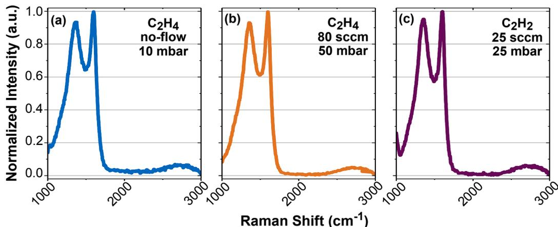
**Figure 3.12:** Comparison of Raman spectra of GC films deposited at different process conditions. All the y-axes have the same scaling. The used precursor gas in (a) and (b) is ethylene with no-flow and flow, respectively, whereas acetylene is used in (c). All have a higher G- than D-peak, only the height of the D-band is slightly different. A difference in the height of second-order peaks is hardly noticeable.
