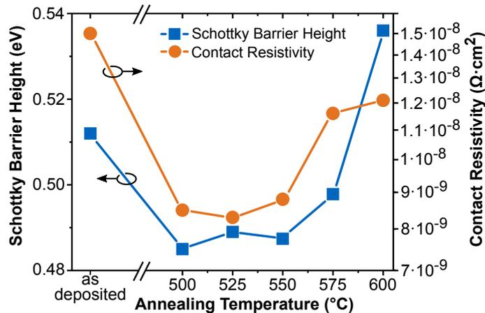
**Figure 1.7:** Schottky barrier height of TiSi on n-Si and contact resistivity of TiSi on n<sup>+</sup>-Si at different annealing temperatures. The doping concentration at the highly doped silicon is  $3 \times 10^{20} \text{ cm}^{-3}$ . The contact resistivity is directly related to the barrier height. An annealing is necessary and the temperature should be  $\leq 550 \text{ }^\circ\text{C}$  to achieve a low  $\phi_B$  and consequently a low  $\rho_c$ . The data are taken from Ref. [30].
