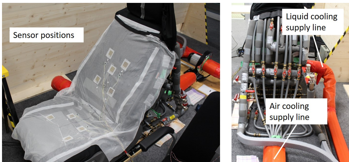
Figure 5.20: Test setup of the seat cooling study.
