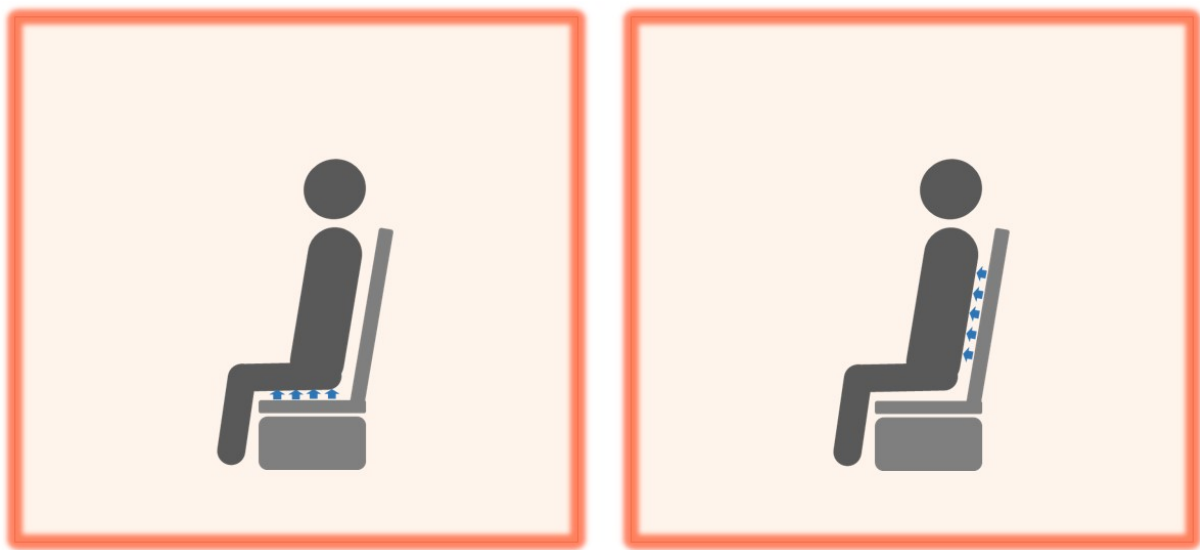
Figure 5.17: Illustration of the test setup for determining TTT_i for the seat (left) and the back (right)
