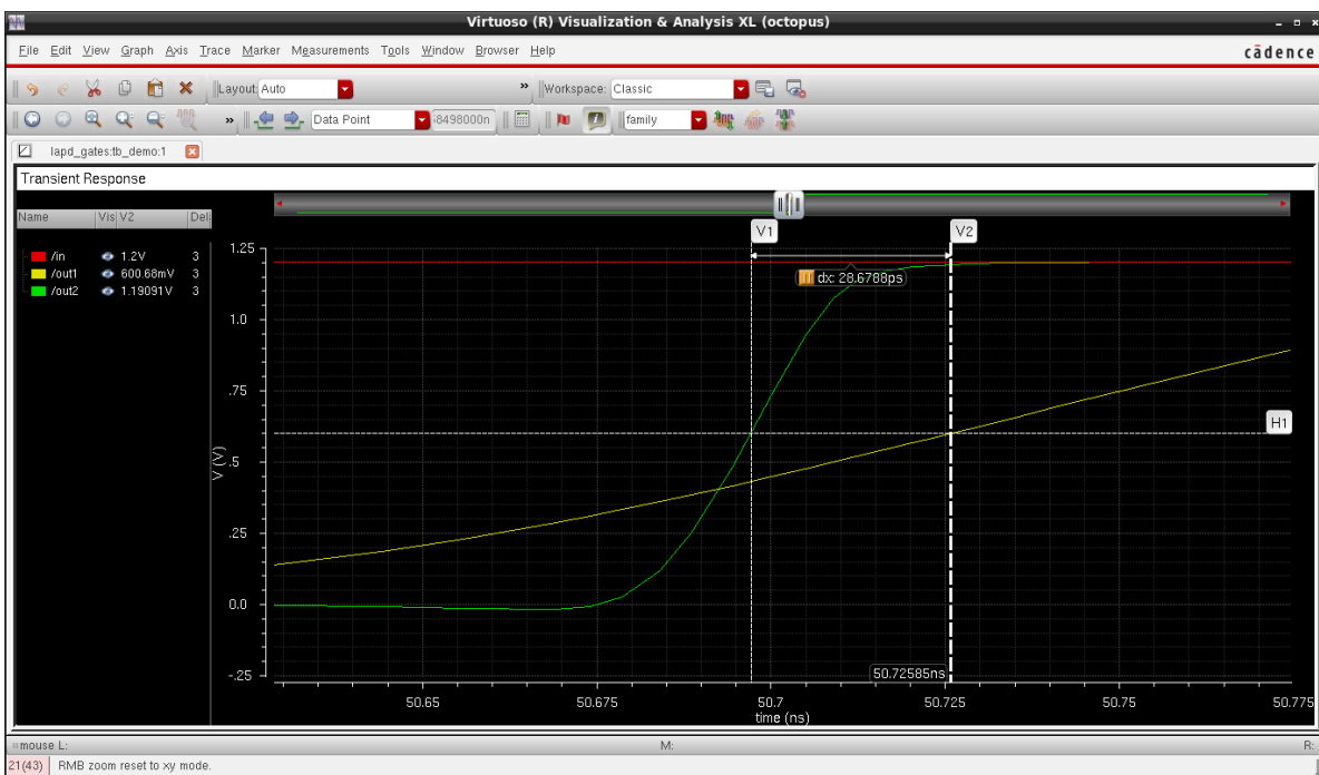
Figure A.8: transient response shown in Virtuoso Visualization & Analysis.
