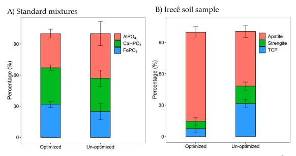
**Figure 4.** Comparison between the LC fit results across the concentrations between 1 to 300 mmol kg<sup>-1</sup> P on the (**A**) standard mixtures and on the (**B**) Irecê soil sample. The selected range includes both a region where self-absorption is neglectable (1 to 75 mmol kg<sup>-1</sup> P) and above the optimum concentration. Note that the results given by the optimized LC fitting are less variable across the different concentrations.
