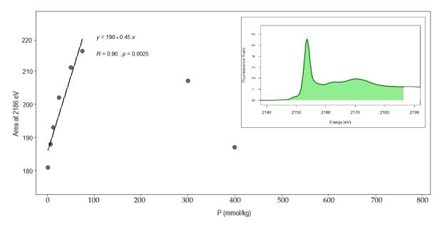
**Figure 1.** Linear correlation between the total P concentration in the standard mixtures (from 1 to 75 mmol  $kg^{-1}$ ) and the absolute area of the spectrum until 2186 eV (colored area). After 75 mmol  $kg^{-1}$  the correlation between concentration and area is not linear anymore, indicating that the spectra were damped by self-absorption.
