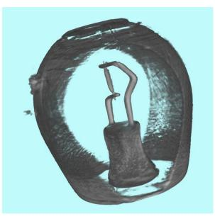
Figure 16. Cut-open 3D view of the optical CT of the light bulb.
