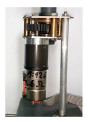
Figure 12. Stepper motor with reduction gear.
