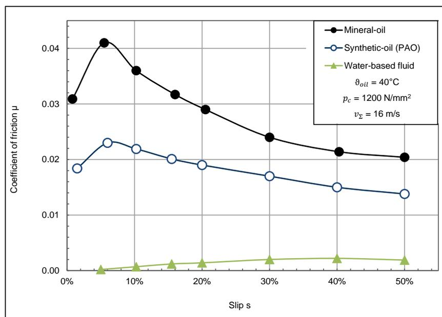
Figure 6. Coefficient of friction of a fluid sample containing water and plant extracts compared to mineral and synthetic oil at 1200 N/mm<sup>2</sup>.
