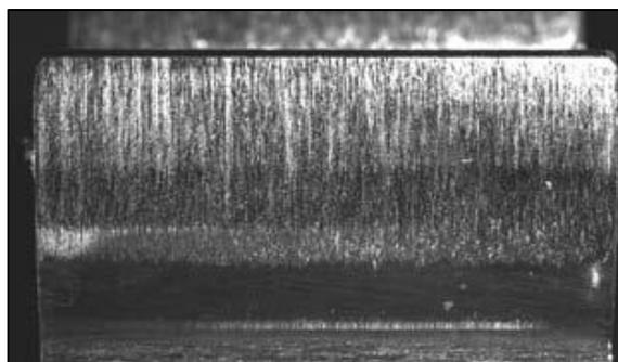
**Figure 8.** Surface of the flank after test, load stage 7.
