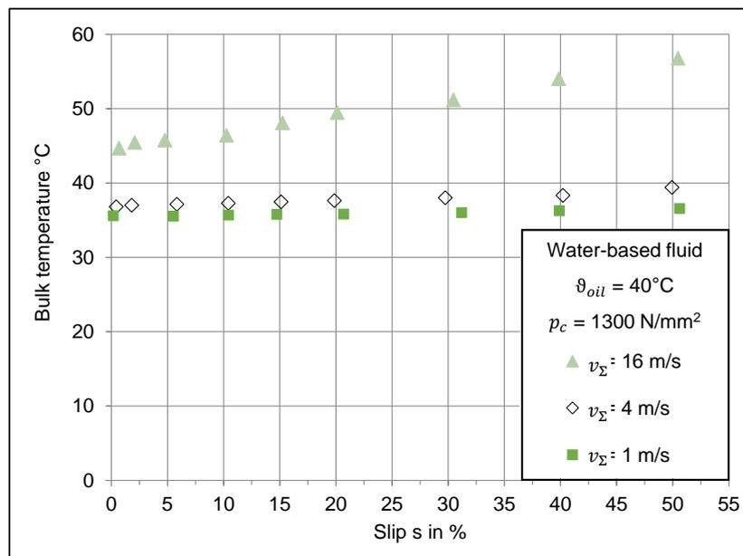
Figure 5. Bulk temperature for a fluid sample containing water and plant extracts at 1300 N/mm<sup>2</sup>.
