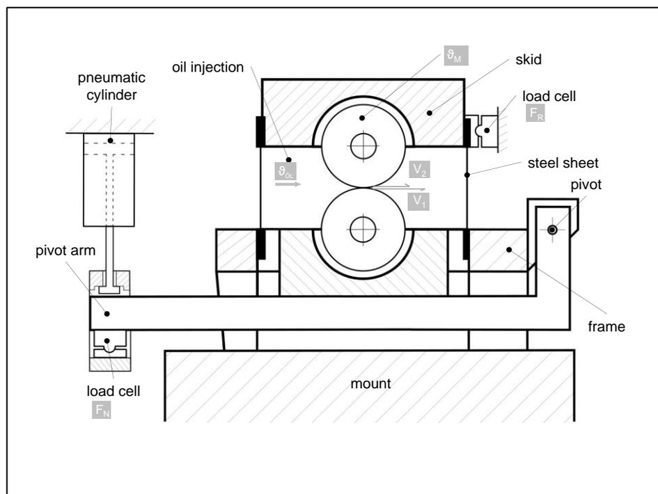
Figure 1. Schematic illustration of the mechanical layout of the considered FZG twin-disk test rig [18].
