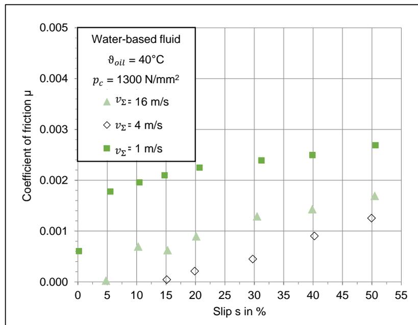
**Figure 3.** Coefficient of friction for a fluid sample containing water and plant extracts at 1300 N/mm<sup>2</sup>.
