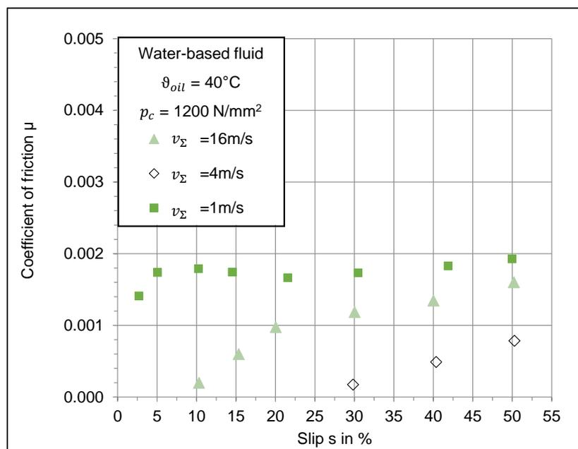
**Figure 4.** Coefficient of friction for a fluid sample containing water and plant extracts at 1200 N/mm<sup>2</sup>.
