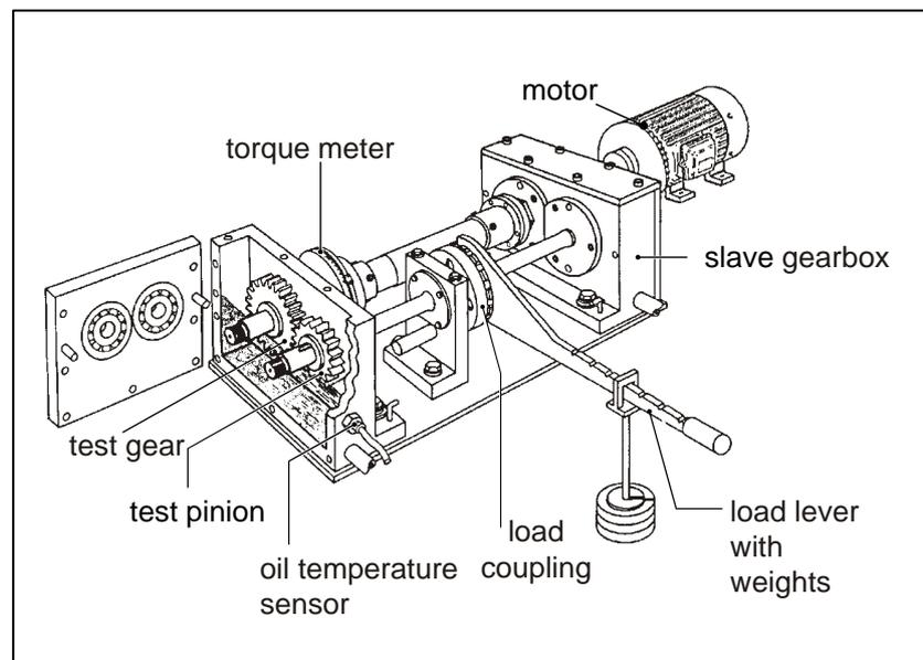
**Figure 2.** Schematic illustration of the mechanical layout of the FZG back-to-back test rig, according to ISO 14635-1 [26].
