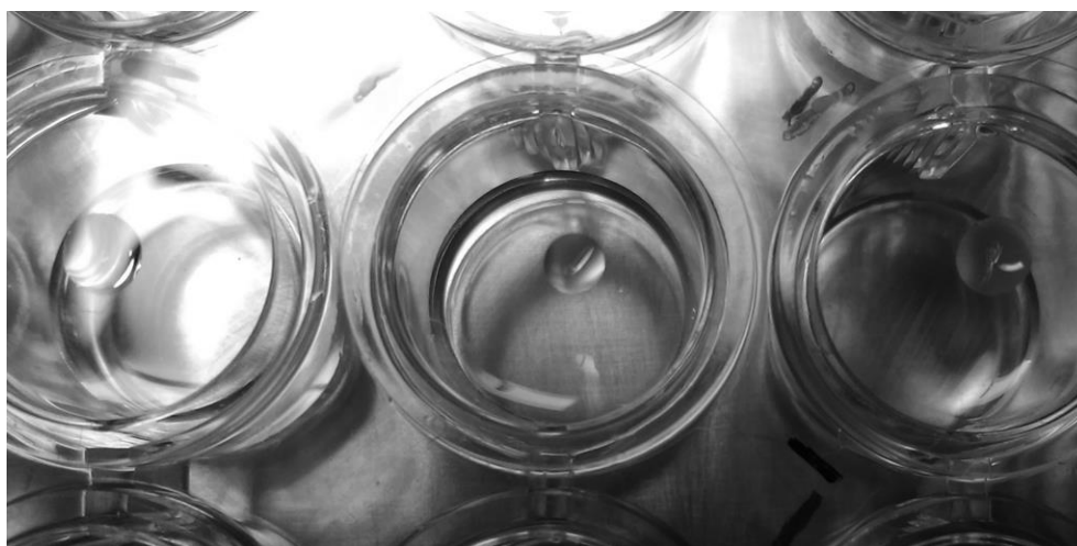
Figure 4.2: Crystallization well of a 24-well vapor diffusion crystallization plate. Inner well diameter = 16 mm. Depicted is the hanging drop technique.
