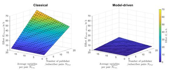
Figure 48: Comparison of implementation efforts for initial deployment as a function of the number of publisher/subscriber pairs and the average number of variables per pair. Classical, manual programming (left), and model-driven approach (right).
