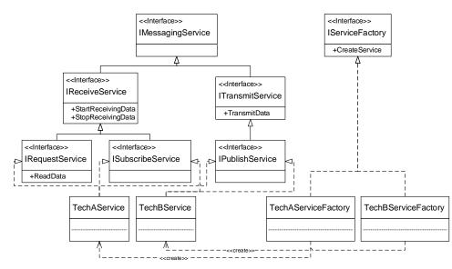
*Figure 31: UML class diagram of the interface definitions for the core software framework. The left part reflects the definition of communication services, right part the service factory definition for dynamic creation of services. Usage of the interfaces shown for two example communication technologies TechA and TechB.*
