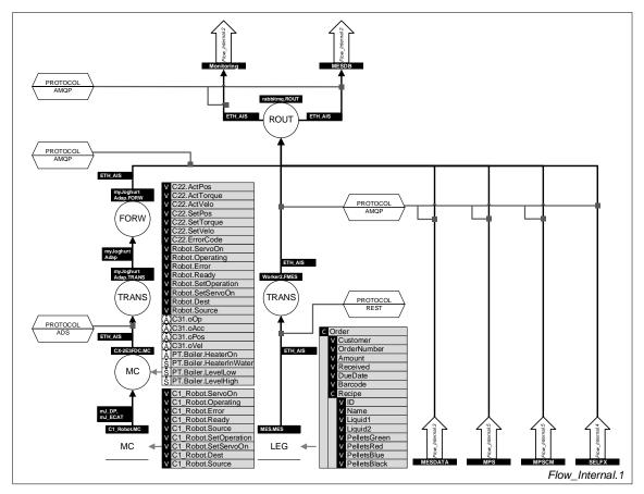
Figure 64: First sheet of the data flow diagram of the internal feasibility study.
