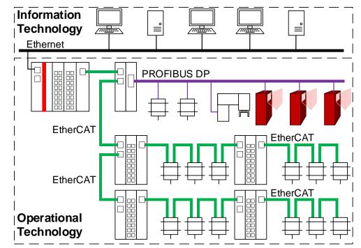
*Figure 6:* Simplified network layout of a typical CPSoS consisting of IT and OT domains with various types of connected devices and networks (Trunzer et al. [TWV20]).
