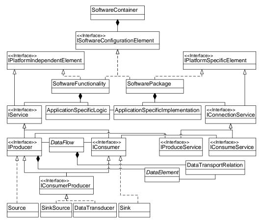
*Figure 24: Detail of the metamodel's SoftwareContainer for the description of the software. Platformindependent part (left) and platform-specific part (right) allow the description at distinct lev els of abstraction.*
