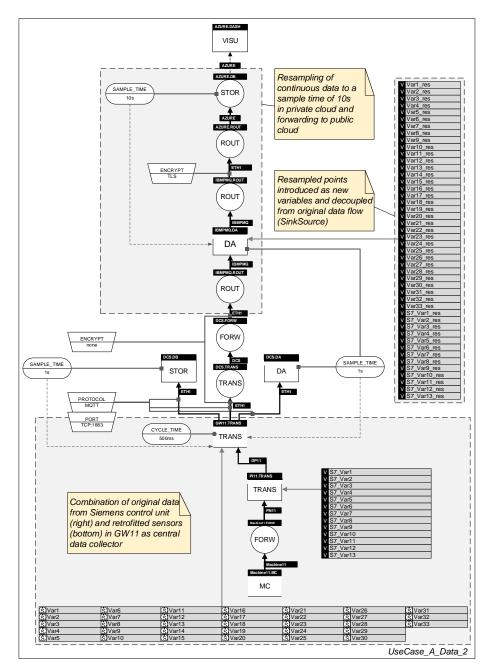
Figure 45: Data flow diagram of Use-Case A with the description of continuous data.
