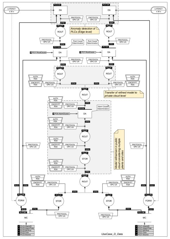
*Figure 60: Alarm management system of Use-Case D modeled in the data flow viewpoint (adapted from [TWV20]). Model refinement based on data from multiple sources (center) and subsequent execution of pre-trained models to diagnose machines.*
