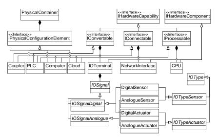
Figure 26: Detail of the metamodel's PhysicalContainer for a description of the system. Physical systems (left) are composed of distinct components (right). IOTerminals may encompass signals (bottom).
