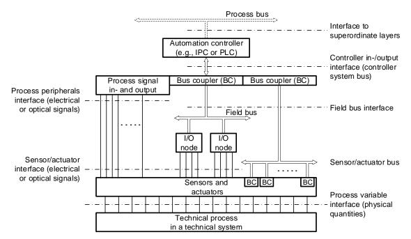
Figure 4: Installations for coupling an automation controller with a technical process, including relevant interfaces (adapted from Lauber and Göhner [LG99b] and VDI/VDE guideline 3687 [VDI3687]). A direct connection between sensors/actuators and automation controller (left), field bus connection using a bus coupler and decentralized I/O nodes (middle), and decentralized intelligent sensors with direct bus access (right).
