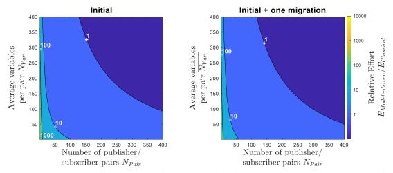
*Figure 52:* Relative effort between model-driven approach and classical, manual programming, including the effort for the creation of the toolchain as a function of the average number of variables per pair. Only initial deployment (left), including one migration (right). Logarithmic scale of the colormap.
