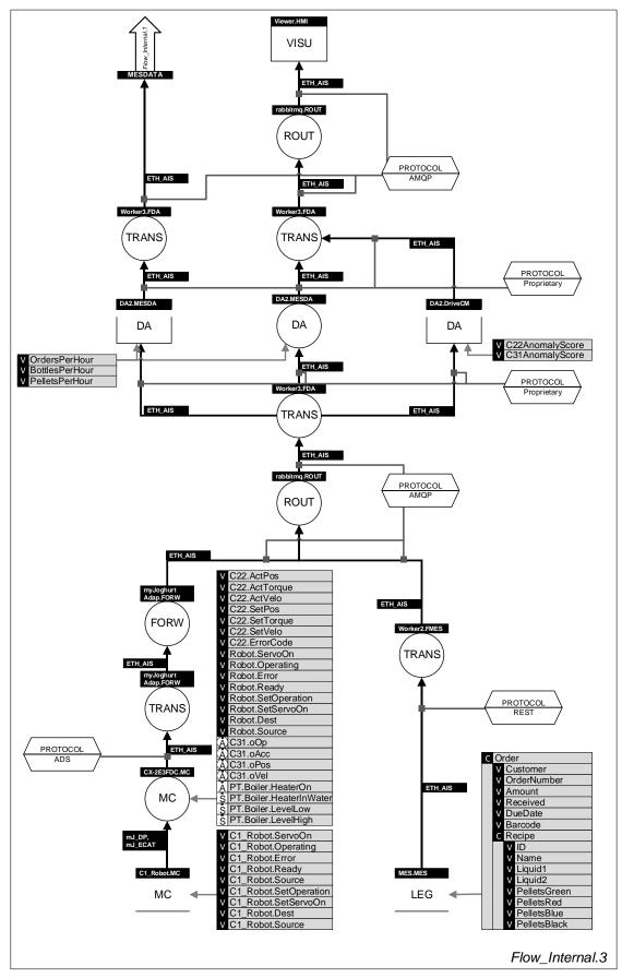
Figure 66: Third sheet of the data flow diagram of the internal feasibility study.
