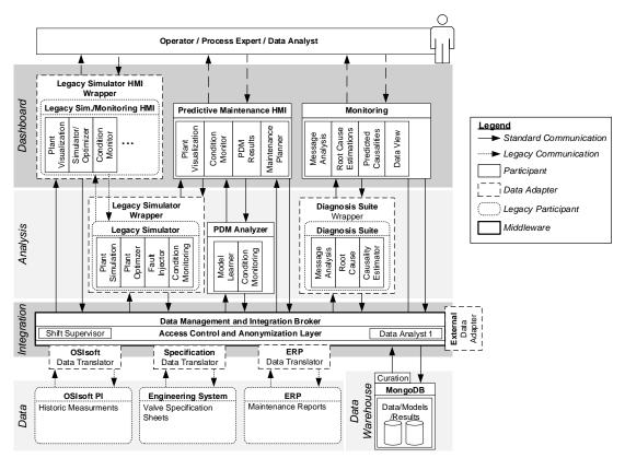
*Figure 39: Representation of the conceptualized architecture for the SIDAP use-case (graphically adapted from Trunzer et al. [Tru<sup>+</sup>17]).*
