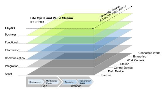
*Figure 7:* Graphical representation of the Reference Architecture Model Industrie 4.0 (RAMI4.0) (DIN SPEC 91345 [DIN91345]) (Trunzer et al. [Tru<sup>+</sup>20b]).
