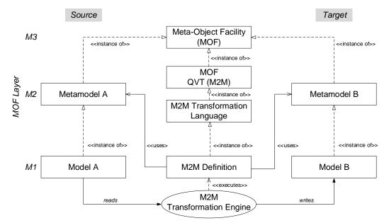
Figure 13: Principle of a model to model (M2M) transformation using a MOF QVT-compliant transformation language (following the conventions from Brambilla et al. [BCW17]).
