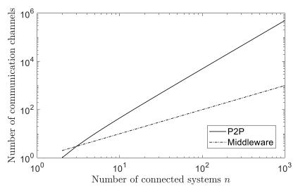
*Figure 20:* Number of necessary communication channels for transparent data access as a function of the number of connected systems n for a fully connected mesh (P2P) and a middleware network.
