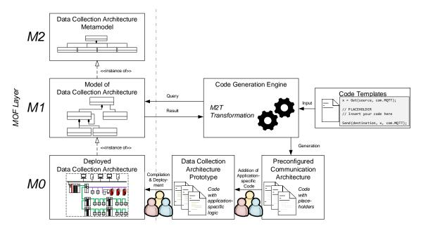
Figure 32: Overview over the process of transforming the model of the data collection architecture to a deployed instance via code generation and addition of application-specific code (adapted from Brambilla et al. [BCW17]). The left side reflects the different models and the related MOF layers. The right side illustrates the process of automatic generation of the communication architecture on OSI layer 7, as well as the addition of application-specific code and the deployment by experts.
