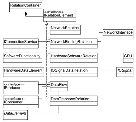
Figure 29: Detail of the metamodel for mapping software (left) and system (right) description with IRelationElements.
