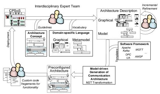
Figure 18: Workflow for model-driven development of data collection system architectures.
