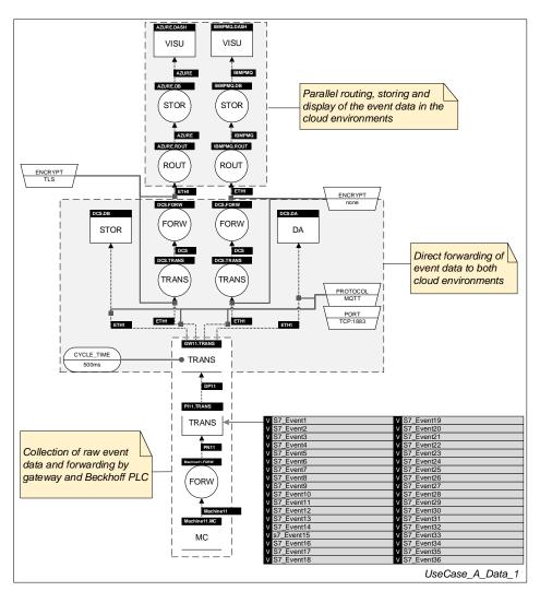
Figure 44: Data flow diagram of Use-Case A with the description of event-based data.
