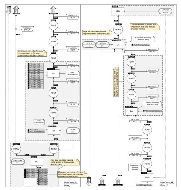
*Figure 56: Data flow of Use-Case B modeled in the data flow viewpoint (adapted from [TWV20]). The diagram is distributed over two sheets for better overview, arrows link the two sheets.*
