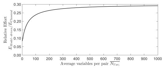
*Figure 49: Relative effort between model-driven approach and classical, manual programming for initial deployment as a function of the average number of variables per pair.*
