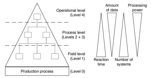
*Figure 5:* Automation pyramid structure and requirements for the communication and processing system (adapted and extended from Scherff et al. [SHW99] and Lauber and Göhner [LG99b]).
