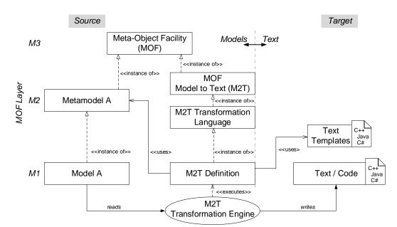
Figure 14: Principle of a model to text (M2T) transformation for text/code generation using a MOF M2T-compliant transformation language (adapted from Aicher [Aic18], as well as Schütz [Sch15] and extended, following the conventions from Brambilla et al. [BCW17]).
