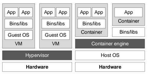
Figure 15: Comparison of virtualization architectures. Layers of hypervisor (left) and container (right) virtualization (adapted from Pahl [Pah15]).
