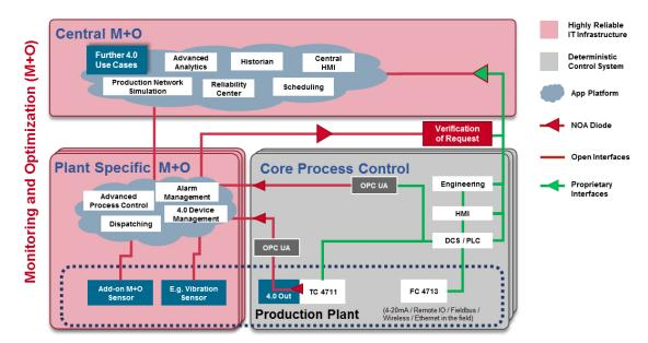
*Figure 8: Concept of the NAMUR Open Architecture (NOA) as a supplement to the existing ISA-95 automation structure (NAMUR NE175 [NE175]).*
