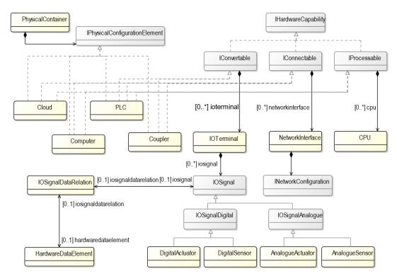
*Figure 33: Excerpt of the metamodel modeled with the Eclipse Modeling Tools showing the PhysicalContainer (cf. Figure 26).*
