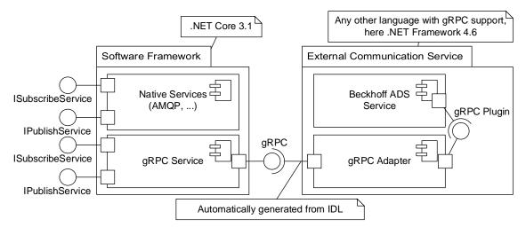
*Figure 35:* Working principle of the flexible extension mechanism via gRPC. Example of Beckhoff ADS support as an external communication service.
