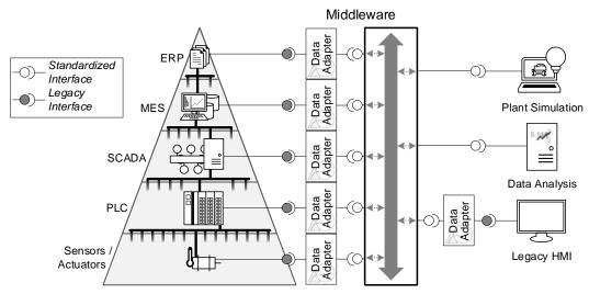
Figure 19: High-level concept of the data collection architecture.
