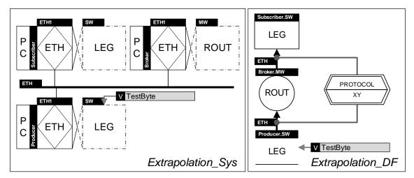
*Figure 47:* System and data flow of the minimal extrapolation use-case modeled with the graphical modeling notation. The protocol specification (requirement) as a placeholder labeled with XY is to be replaced by the specific protocol.
