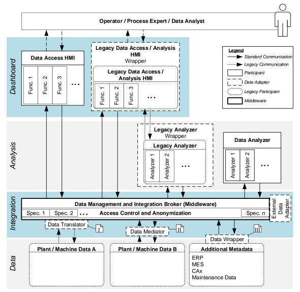
*Figure 21: Detailed concept of the data collection architecture (adapted from [Tru+19c]).*
