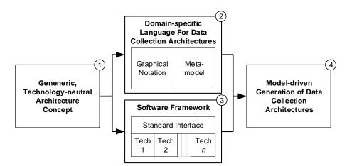
*Figure 17:* Building blocks of the concept. Generic, technology-neutral architecture concept (left, 1), the domain-specific language for data collection architectures including the graphical notation and the metamodel (top, 2), the software framework for different communication technologies (bottom, 3), and the model-driven generation of the data collection architecture (right, 4).
