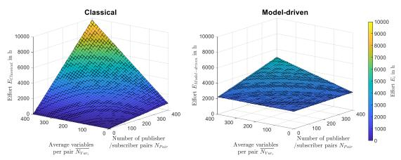
*Figure 51:* Comparison of implementation efforts for an initial deployment, including the effort for the creation of the model-driven toolchain as a function of the number of publisher/subscriber pairs and the average number of variables per pair. Classical, manual programming (left), and model-driven approach (right).
