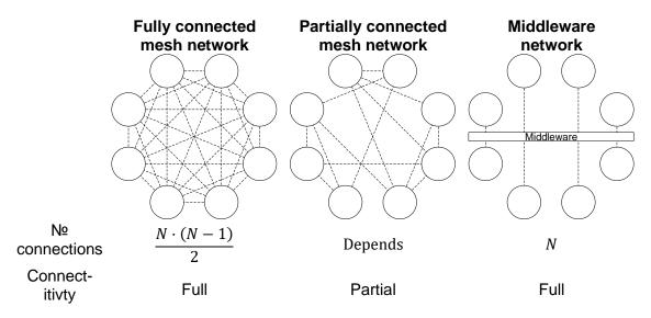
Figure 11: Comparison of different network structures with the number of connections depending on the number of systems N and connectivity [Haa97; Ind17c].
