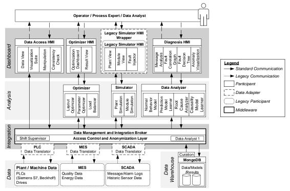
*Figure 40:* Representation of the conceptualized architecture for the IMPROVE use-case (graphically adapted from Trunzer et al. [Tru<sup>+</sup>17]).
