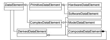
Figure 25: Detail of the metamodel for the description of DataElements.
