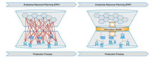
*Figure 10:* Information diabolo with individually engineered, direct P2P connections (left) and with a common information model (right) (Vogel-Heuser et al. [Vog<sup>+</sup>09]).
