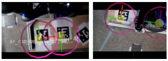
(a) Two markers are fully visible, one is not detected. (b) One marker is occluded by the robot arm.
