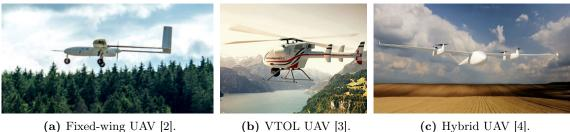
Figure 1.1: Three different classes of unmanned aerial vehicles (UAVs).
