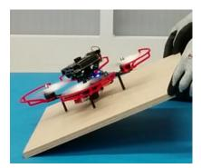
(c) Quadrocopter using downward thrust on a tilted wooden plate.
