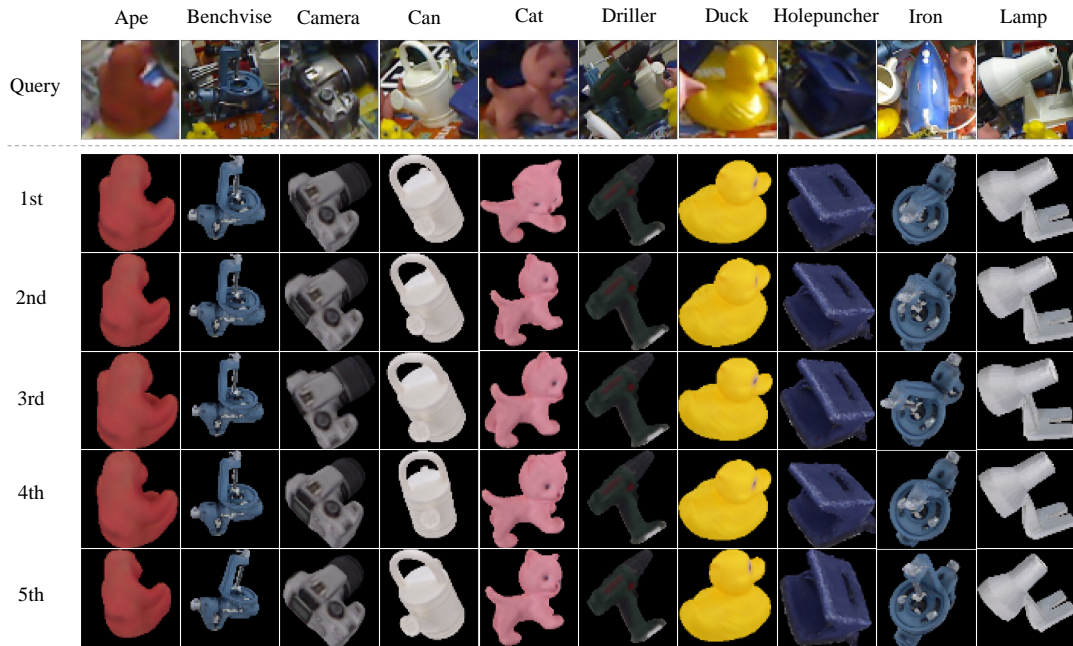
Fig. 4.9. Query patch and its top five retrieved nearest neighbors from the database obtained by our method NNours when trained on RGB information.
