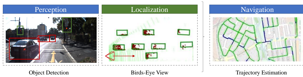
Fig. 1.1. Perception of the vehicle’s environment and its localization are core requirements for autonomous control and navigation. Images are adapted from the KITTI Dataset [70].
