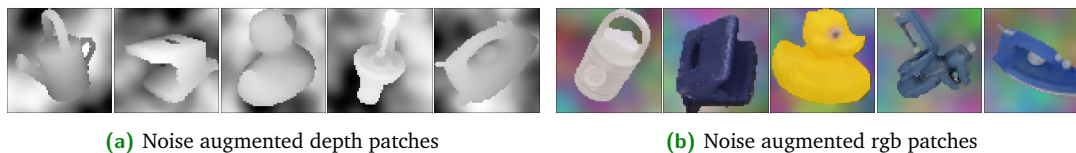
Fig. 4.4. Example depth and RGB renderings with augmented noise as background information.
