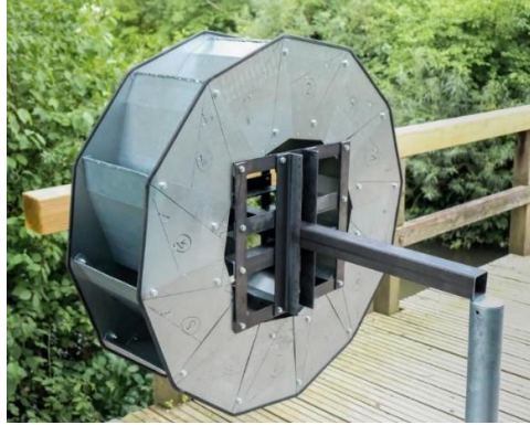
Figure 1 Overshot wheel fabricated by Lukas Geb and Johannes Eisner in Germany [6]
