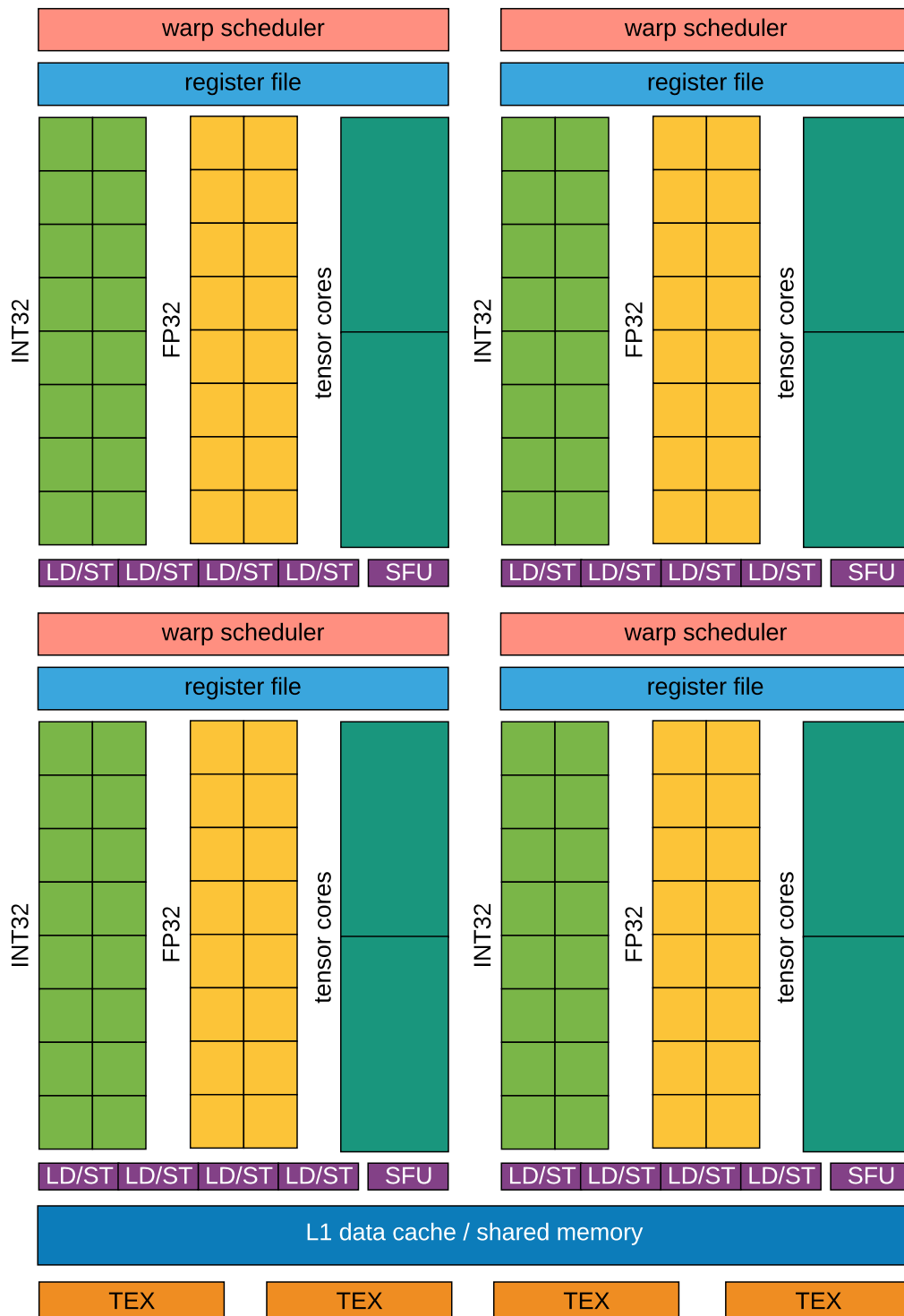
Figure 2.1.1: Schematic of a Streaming Multiprocessor (SM) of the Turing GPU architecture based on the NVIDIA whitepaper [17].
