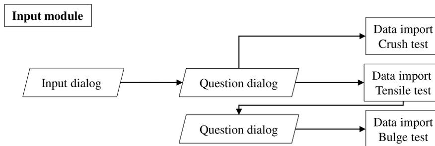
Fig. 2. Architecture of MaterialModeler input module.
