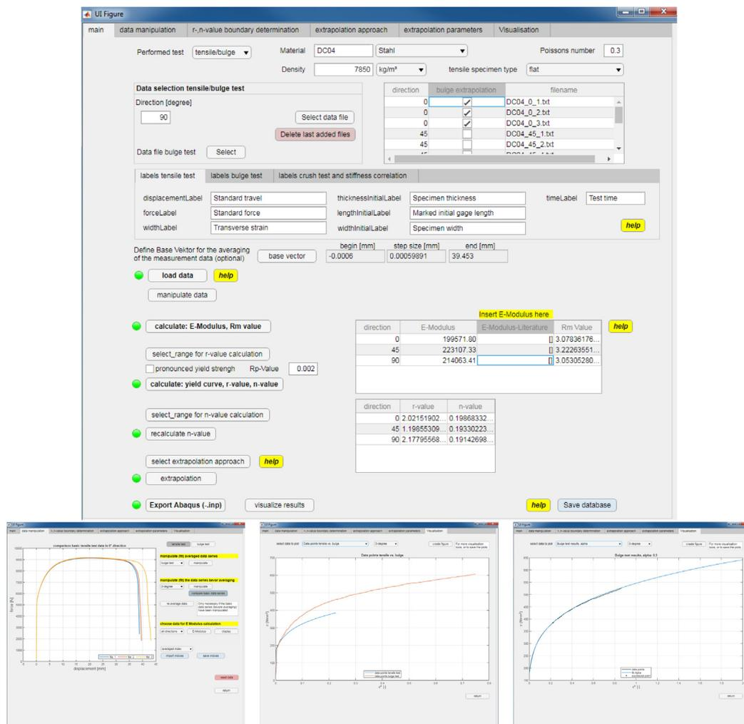
Fig. 4. Overview of MaterialModeler's GUI (top); unprocessed experimental raw data (left); processed experimental data from tensile and bulge tests (middle); final material model (right).
