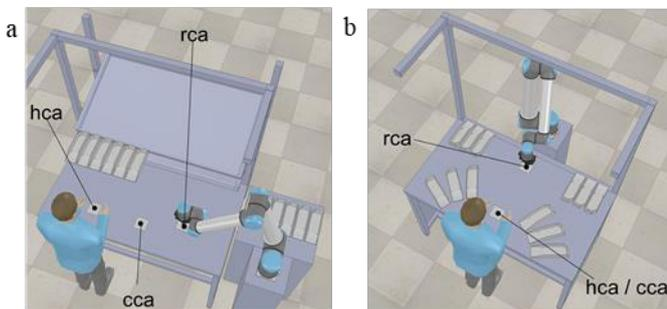
Fig 3: (a) distinguished centers of assembly, (b) combined centers of assembly
