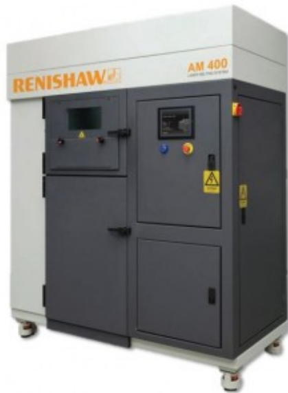
(a) Selective Laser Melting metal 3D printer (Renishaw AM400) located in the laboratories of the University of Pavia ( http://www-4.unipv.it/3d/laboratories/3dmetalunipv/ ).
