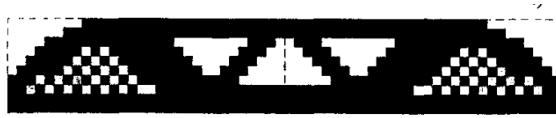
Figure 6.1: Example of checkerboard pattern for simply supported beam problem from Sigmund and Petersson [1998].
