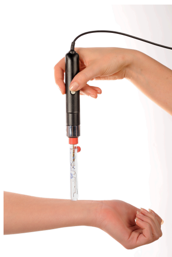
Figure 2.4 The pH-meter probe. The glass probe is held in 90 degree angle to the area of the skin one would like to measure, shown in the image is a measurement of the lower part of the arm. Figure retrieved from the Courage and Khazaka website ( https://www.courage-khazaka.de/de/downloads/item/foto-probes-ph-arm ; 04.01.2019; downloaded 04.11.2019).
