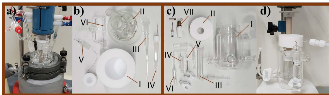
Figure 13. a) Cell setup and b) individual components for RDE measurements in alkaline solution. c) Components and d) cell setup for acid solution. The hardware consists of I) an electrolyte reservoir, II) a lid, III) an electrolyte bridge / Luggin capillary, IV) a reference electrode, V) a counter electrode, VI) a bubbler and VII) an electrode holder with electrode.
