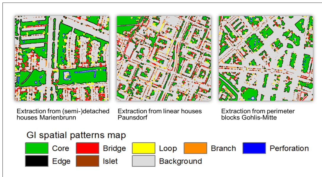
Figure 17. GI spatial patterns map in three types of the residential area (Wang et al., 2019a)
