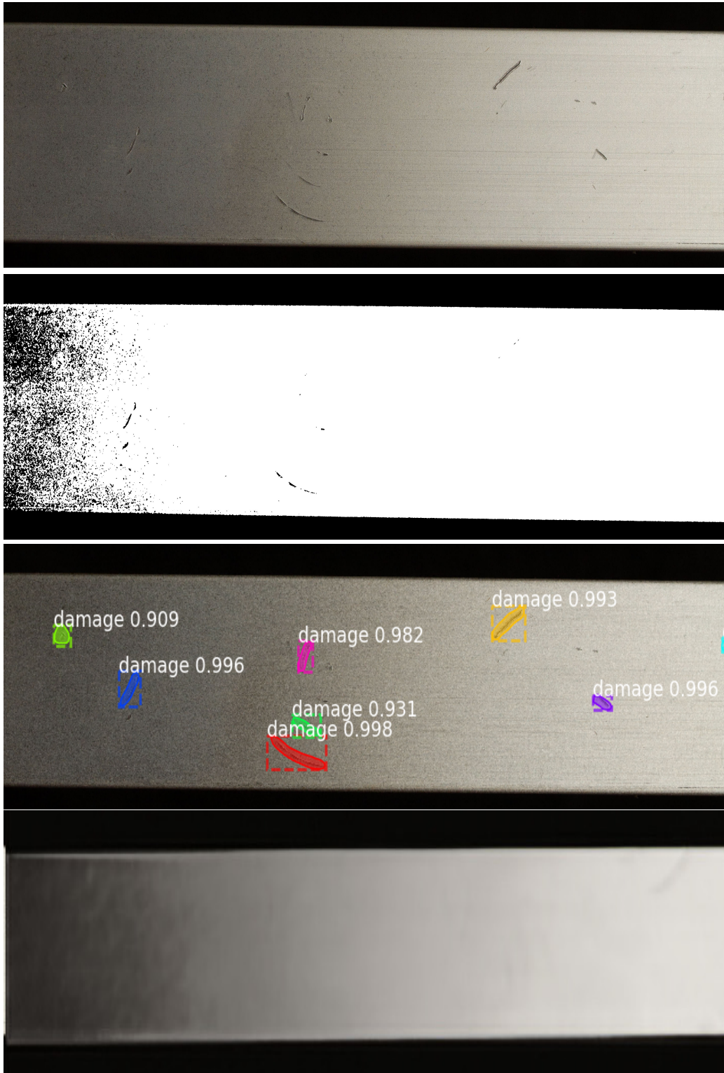
Figure 4.7: An example of the original image input (first row), thresholding result (second row), segmentation result using Mask R-CNN (third row), and its autoencoder reconstruction (last row) for aluminum surfaces.
