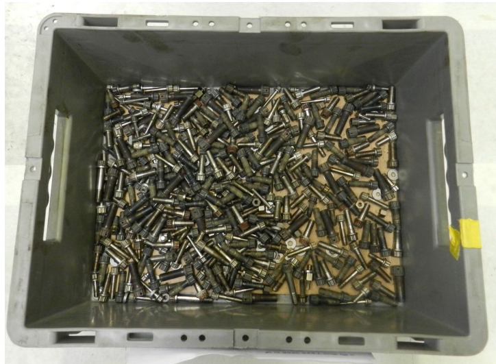
Figure 1.9: Fasteners that were taken from part of engine and must be classified during inspection in overhaul process.
