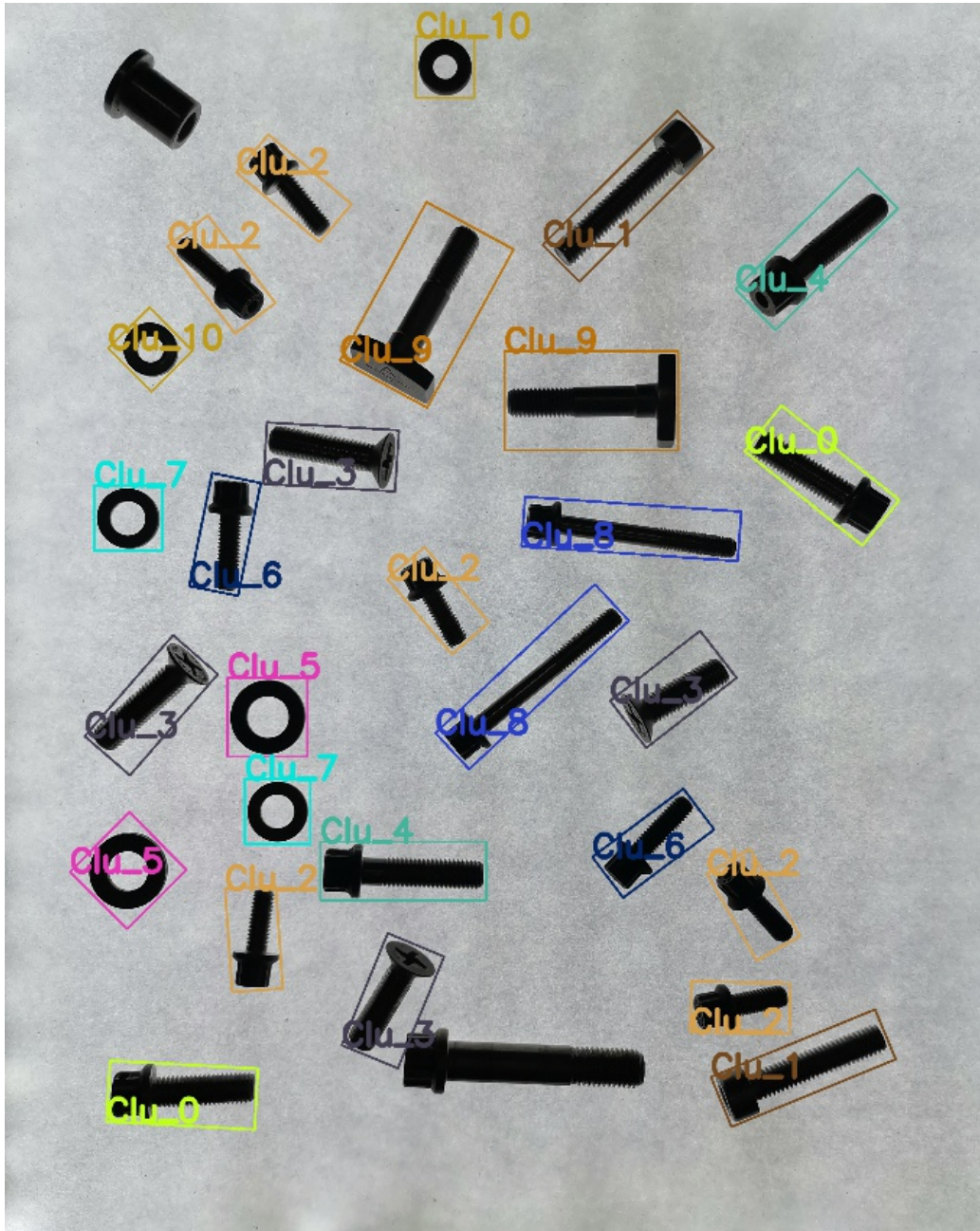
Figure 5.2: The result of computed similarity of the fasteners on the input image (Figure 5.1).
