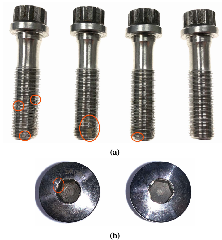
Figure 1.7: Examples of intact and damaged bolts from a side view (a) and top view (b). The annotated damages show either scratches or dirt which could not be cleaned by washing [Taheritanjani et al., 2019b].
