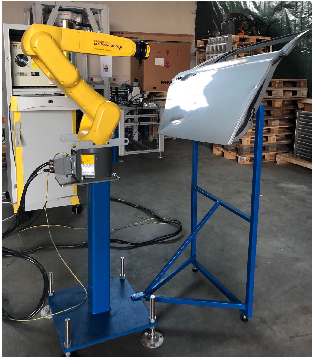
Figure 8.11: The hardware platform used in SUMA . The robotic arm is equipped with a 3D camera and sees the surface in front of it.
