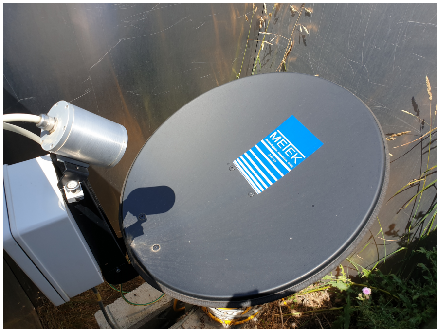
Figure 1.3: Micro rain radar (MRR) located in Das, north east of Spain. Photo by Ghada, Wael. (2019)
