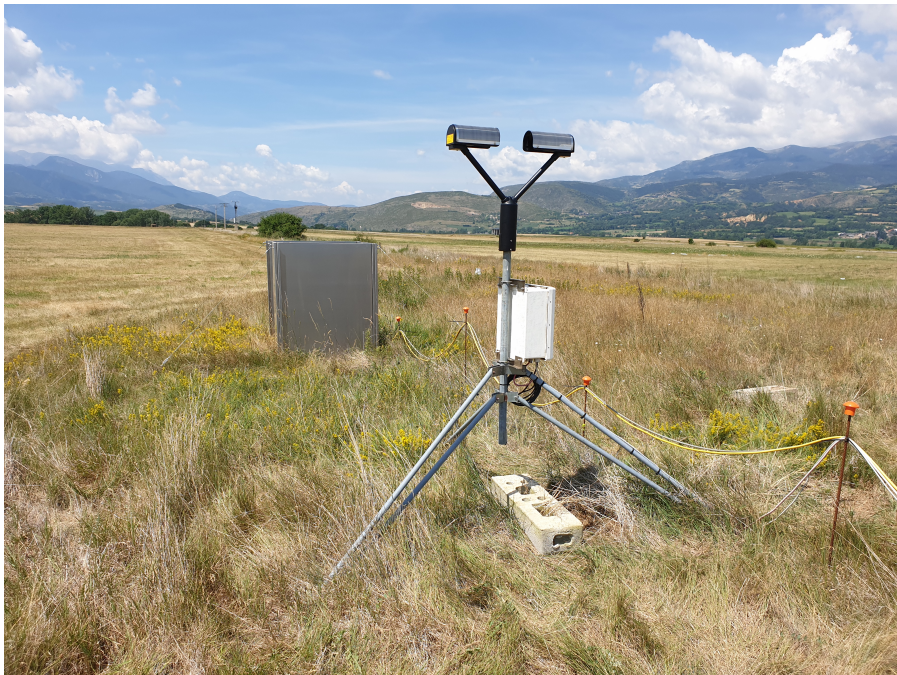
Figure 1.2: The PARSIVEL disdrometr (front) and the micro rain radar inside its housing (back) located in Das, north east of Spain. Photo by Ghada, Wael. (2019)
