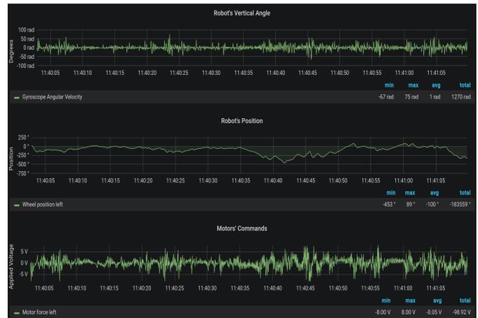
Fig. 3: Time evolution of the QoC KPIs: motors' commands (bottom), robot's position (mid) and vertical angle (top).
