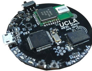
Figure 6.9: Hardware prototype of UWB-equipped smartwatch
