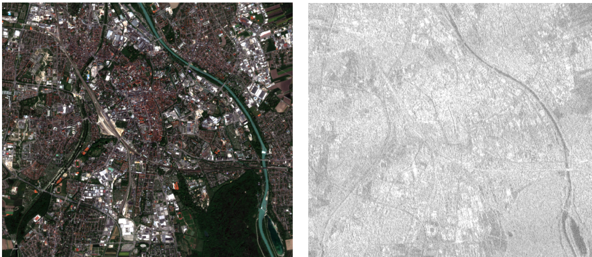
Fig. 2.2. A visualization of an optical image and a SAR image of the same scene, the city of Augsburg, Germany. The optical image is a Sentinel-2 image with red-green-blue channels. The SAR image is a Sentinel-1 intensity image in dB.
