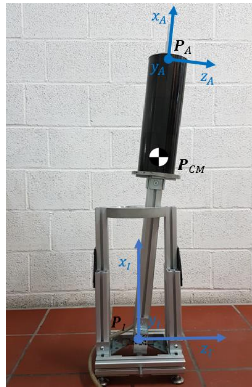
Fig. 3-6: Test stand with the inertial coordinate frame, I , and the actuator coordinate frame, A . Actuators not mounted.
