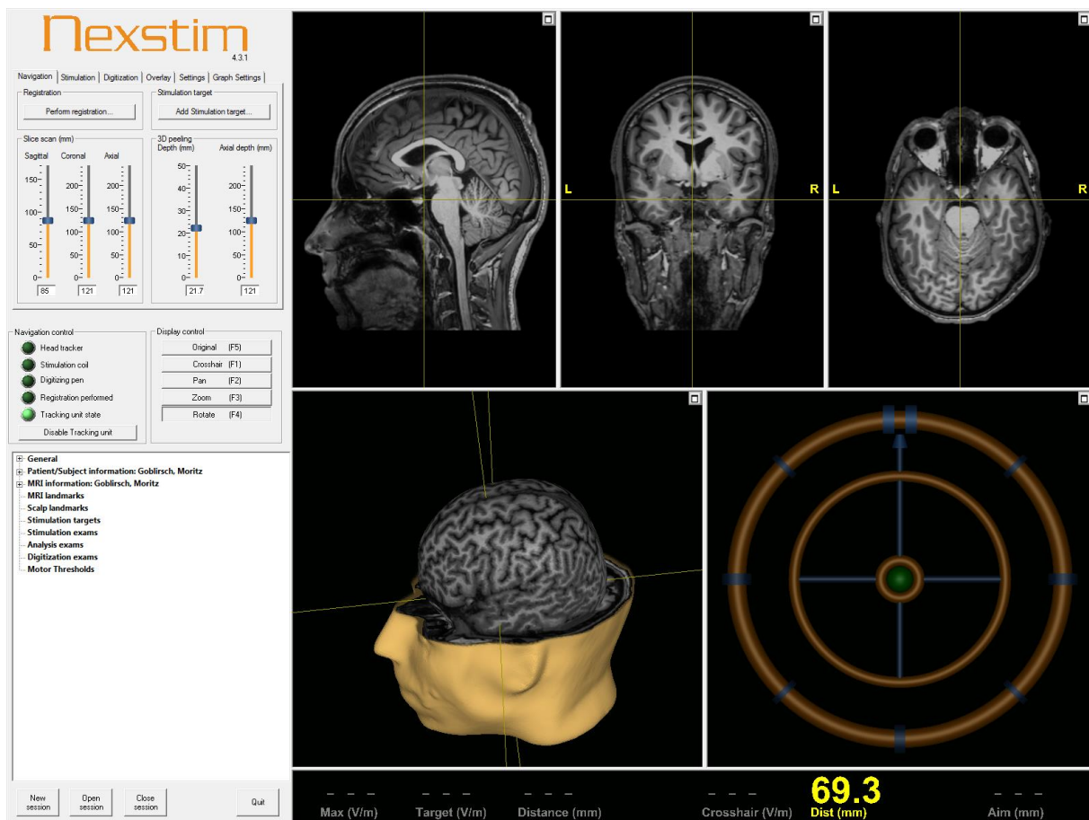
Figure 8 Display of the EnTMS device's software after import of a healthy subject's (non-contrast-enhanced) MRI. Note the first row with the original sagittal, coronal and axial scans on the top and the computed 3D model on the bottom left. Peeling depth was set to 21.7 mm on the left side control.
