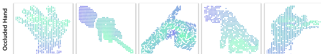
Figure 3.5: Project depth images to final occluded hand point clouds. Brightness indicates depth value, namely, darker point denotes that the point is more distanced to camera, and vice versa.
