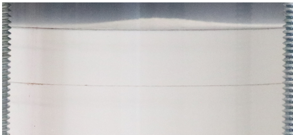
Fig. 6.22.: Top surface of the bed after lateral vibration with 2 K-8 vibrators at 4 bar.
