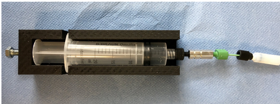
(a) 3D-printed syringe adapter for the manual packing and pumping of PEEK capillaries. A green capillary can be seen attached to the end of the syringe
