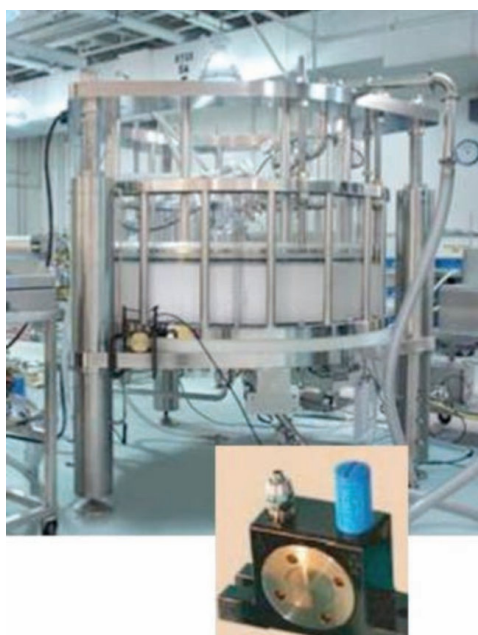
(a) Turbine rotational vibrator clamped to column flange for packing of irregular silica or controlled pore glass [5].
