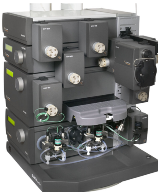
(b) ÄKTA Purifier ©HPLC (GE-Healthcare) station employed for the packing and preparation of final samples of PEEK capillaries.
