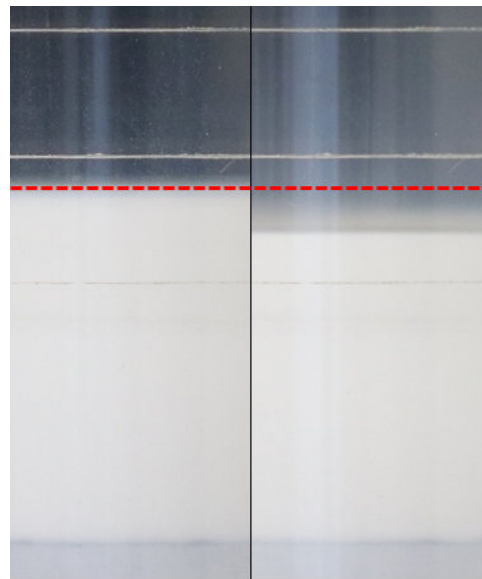
(b) CHT bed (left) after flow-packing, and (right) after vibration (compaction = 13%). Red dashed line indicates initial bed height of \sim 25 mm.
