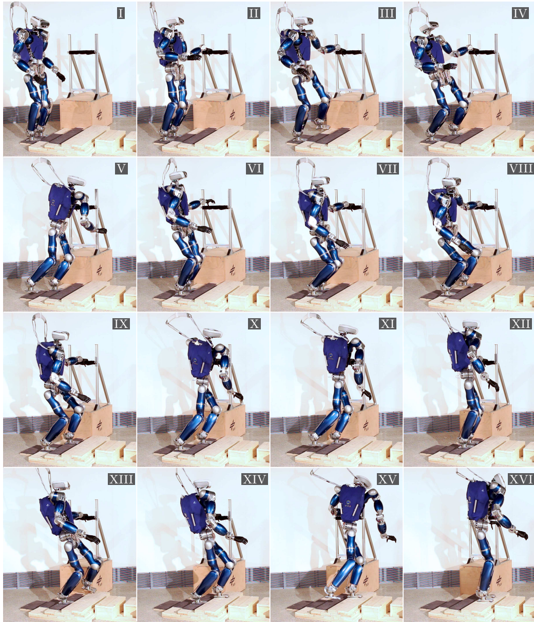
Figure 9.4: The humanoid robot TORO climbing stairs with a height of 5 cm.
