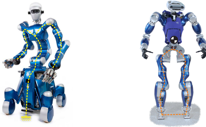
(a) Humanoid robot Rollin' Justin featuring a serial kinematic chain originating from a fixed base.
