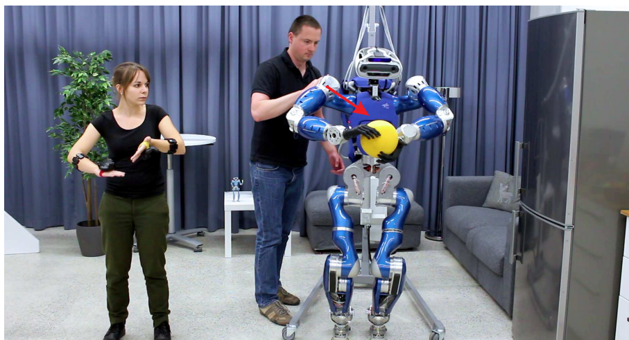
(a) Bimanual handling of a ball while balancing compliantly in the presence of external disturbances (red arrow).
