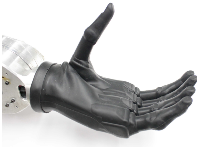
(a) Left hand of the humanoid robot TORO .
