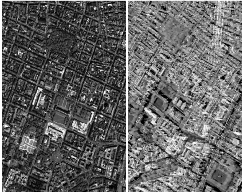
Figure 6. Display of SAR-optical sub-scenes extracted from Munich study areas (the left-hand image is from WorldView-2, the right-hand image is from TerraSAR-X).
