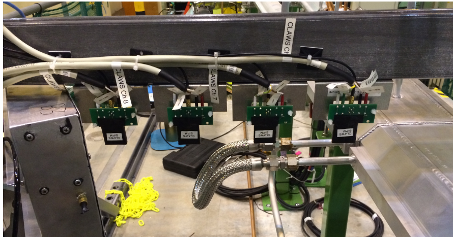
Figure 5.6: Photograph of the CLAWS backward station taken from the position of the IP. Four sensor modules are mounted on the BEAST support structure in the plane of the accelerator with increasing radial distance from the beampipe (shown on the right).
